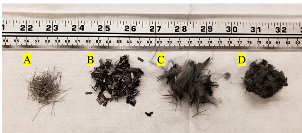
**Figure 1.** Different fiber types mixed into concrete. (A) steel fibers; (B) Hexcel carbon fiber platelets; (C) Zoltek carbon fiber; (D) recycled carbon fiber.
