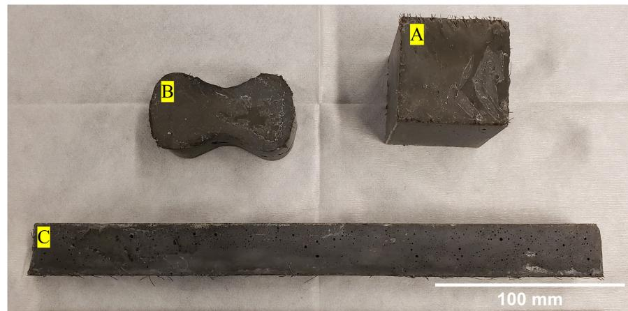
**Figure 2.** Different sample types used for mechanical testing. (A) compression cube (50 mm × 50 mm × 50 mm); (B) tension briquettes (at gage 25 mm × 25 mm); (C) flexural beam (25 mm × 25 mm × 305 mm).
