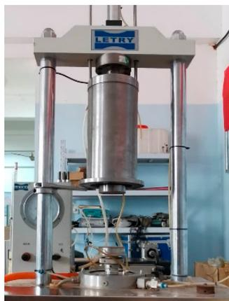
**Figure 2.** The STD-50 triaxial testing apparatus.
