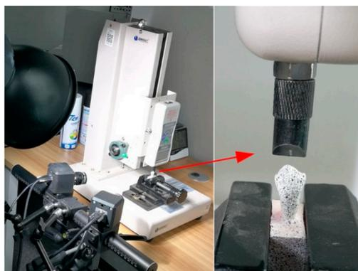
**Figure 2.** Measurement setup. The 3D DIC device monitoring the buccal surface of the specimen that fixed on the fixture of the testing machine.
