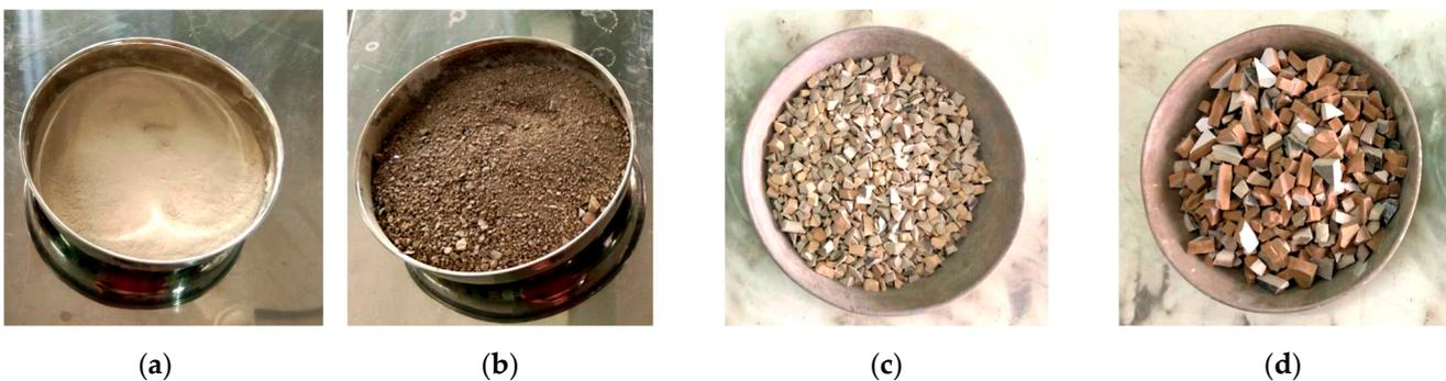
**Figure 3.** (a) Waste ceramic cement ( $C_{WC}$ )—75  $\mu$ m; (b) waste ceramic sand ( $S_{WC}$ )—4.75 mm (c) waste ceramic aggregate ( $A_{WC}$ )—10 mm; (d) waste ceramic aggregate ( $A_{WC}$ )—20 mm.
