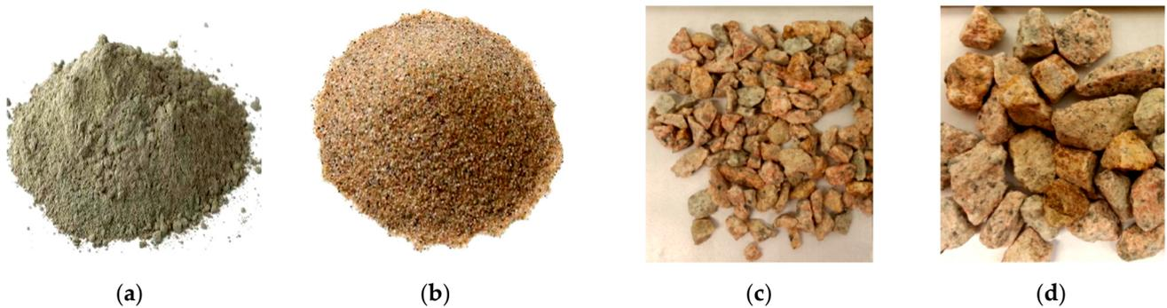
**Figure 2.** (a) Commercial cement; (b) river sand; (c) natural coarse aggregates (NCA)—10 mm; (d) natural coarse aggregates (NCA)—20 mm.
