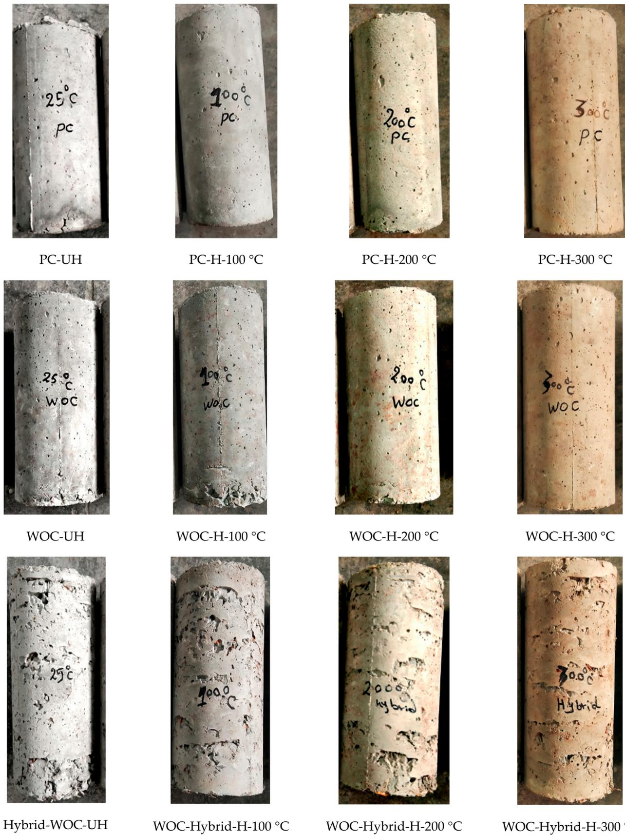
**Figure 8.** PC, WOC, and WOC-Hybrid specimen colour after being exposed to 100 °C, 200 °C, and 300 °C.
