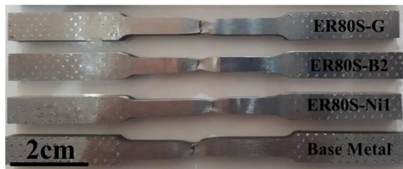
Figure 11. Tensile test specimen showing the necking and fractured regions.
