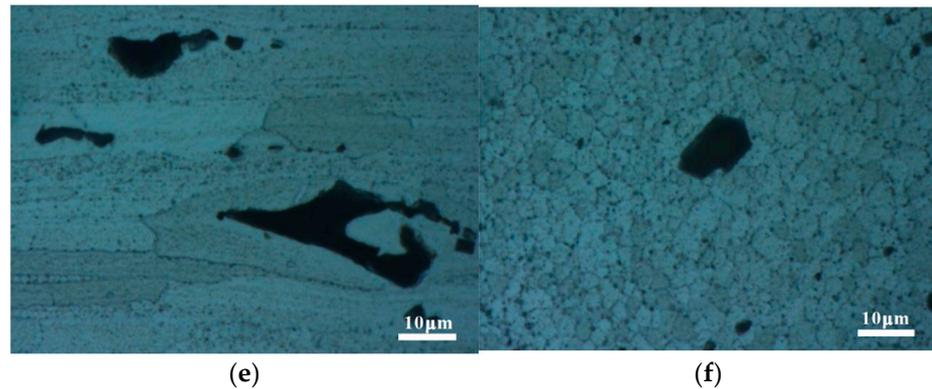
**Figure 5.** Microstructure of the 7050 aluminum alloy's FSW joints: (a) the TMAZ-SZ; (b) the HAZ; (c) high-magnification morphology of the TMAZ-SZ; (d) secondary-phase morphology of the HAZ; (e) secondary-phase morphology of the SZ; (f) SEM of the BM.
