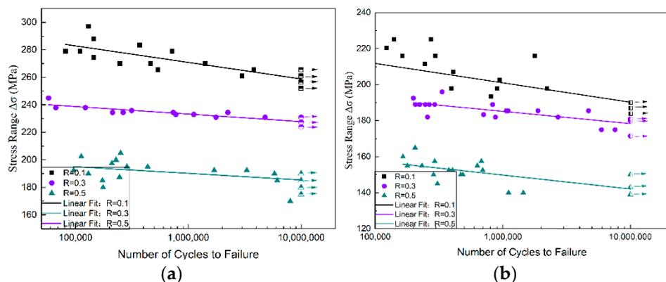
**Figure 4.** Fatigue S–N curves of the BM and FSW joints: (a) fatigue S–N curves of the BM subjected to  $R = 0.1$ ,  $0.3$ , and  $0.5$ ; (b) fatigue S–N curves of the FSW joints subjected to  $R = 0.1$ ,  $0.3$ , and  $0.5$ .
