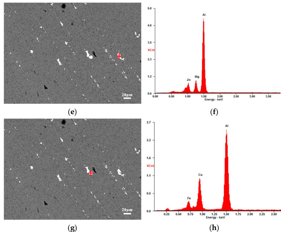
**Figure 6.** EDS spectra of the secondary phases: (a,c,e,g) SEM images of the matrix; (b) Mg<sub>2</sub>Si; (d) Al<sub>23</sub>CuFe<sub>4</sub>; (f) Al<sub>2</sub>Mg<sub>3</sub>Zn<sub>3</sub>; (h) Al<sub>7</sub>Cu<sub>2</sub>Fe.
