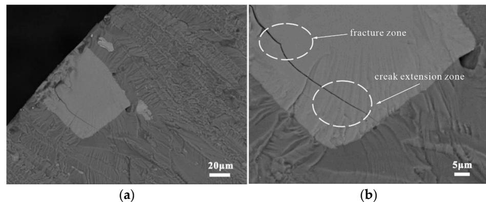
**Figure 13.** Cracking of the non- $Mg_2Si$  phase in joint specimens: (a) origin of the fracture pattern and (b) local magnification.
