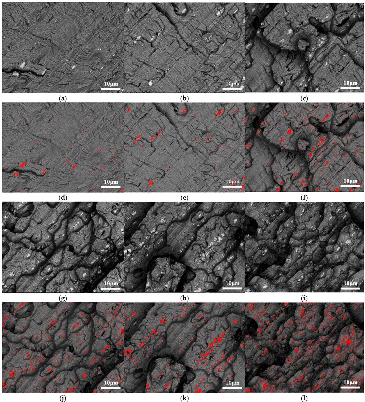
**Figure 14.** Distribution of the coarse secondary phase, during different stages of the fatigue crack extension: (a) early expansion stage; (b) stable expansion stage; (c) boundary between the stable and unstable expansion stages; (g) unstable expansion stage I; (h) unstable expansion stage II; (i) unstable expansion stage III. (d) processed image, (e) processed image, (f) processed image, (j) processed image, (k) processed image, (l) processed image.
