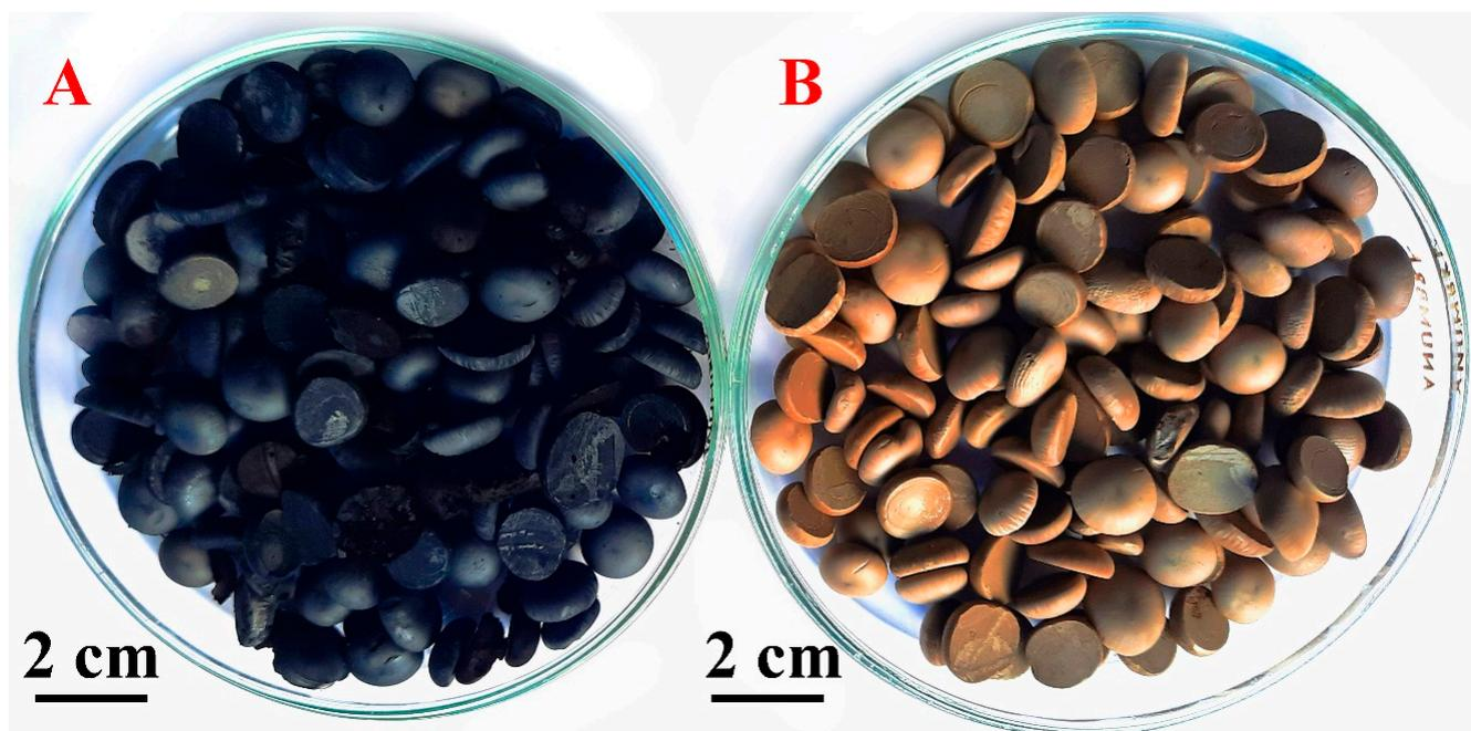
**Figure 1.** Photographs of composite aerogel after reduction (A) and before reduction (B).
