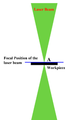
Figure 2. Position of the workpiece surface at the focal position of the laser beam.
