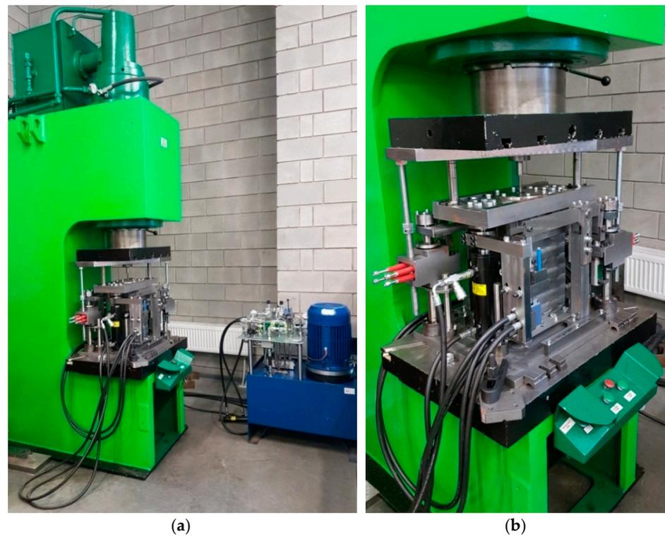
**Figure 4.** Test stand for performing semi-open die extrusion with a moveable sleeve: (a) PYE 160SS hydraulic press provided with a hydraulically driven extruding device, (b) view of the working space of the hydraulic press.
