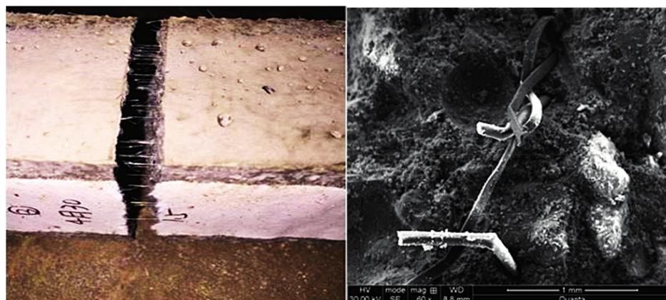
Figure 23. Flexural fracture of coal gangue concrete [108].
