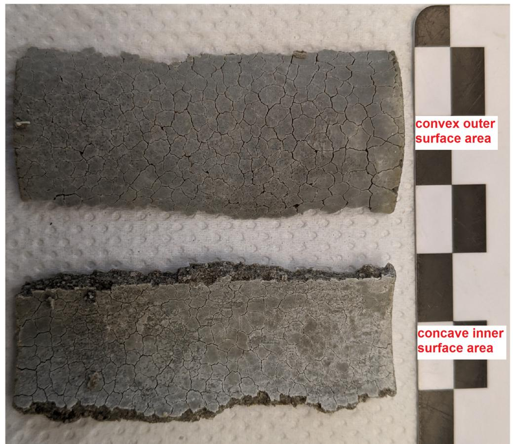
**Figure 10.** Segments of a hollow cylinder (OPC H) at the time of mechanical failure after 38 days (non-constrained stress cell) of storage in 3.0 g L  $\text{SO}_4^{2-}$ .
