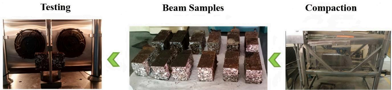
**Figure 5.** Preparation of Three-Point Bending Beam Samples and UTM Setup.
