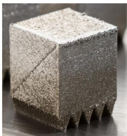
**Figure 2.** Specimen cube with a wedge-shaped support structure.
