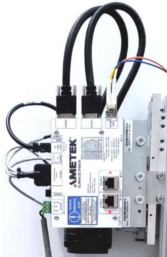
Figure 4. Surface inspection camera with Ametek Camera Link Interface module [31].
