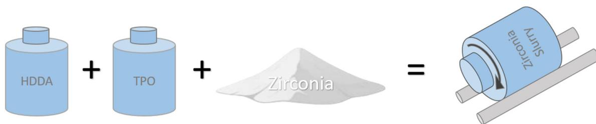
**Figure 3.** Preparation of making zirconia slurry.
