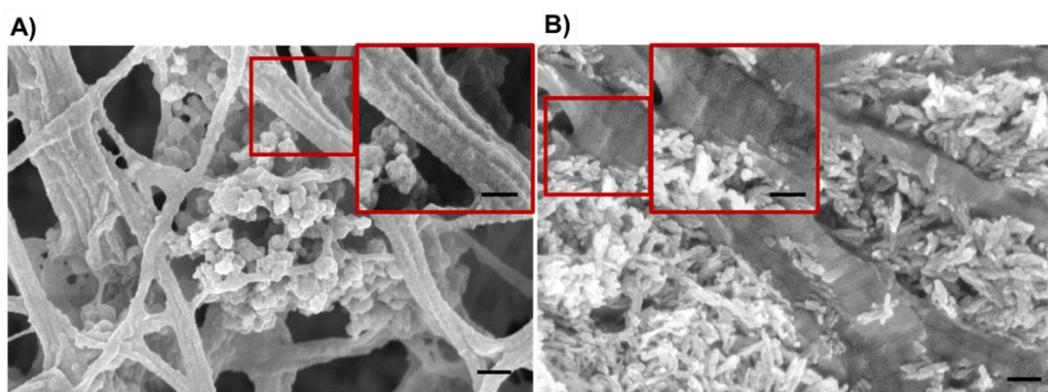
**Figure 10.** FE-SEM micrographs of produced scaffolds after freeze-drying. (A) GEN-Coll/MBG\_Sr4% and (B) GEN-Coll/nanoHA. Collagen D bands seen in both samples and zoomed in on area delimited by the red squares. Scale bar 100 nm.
