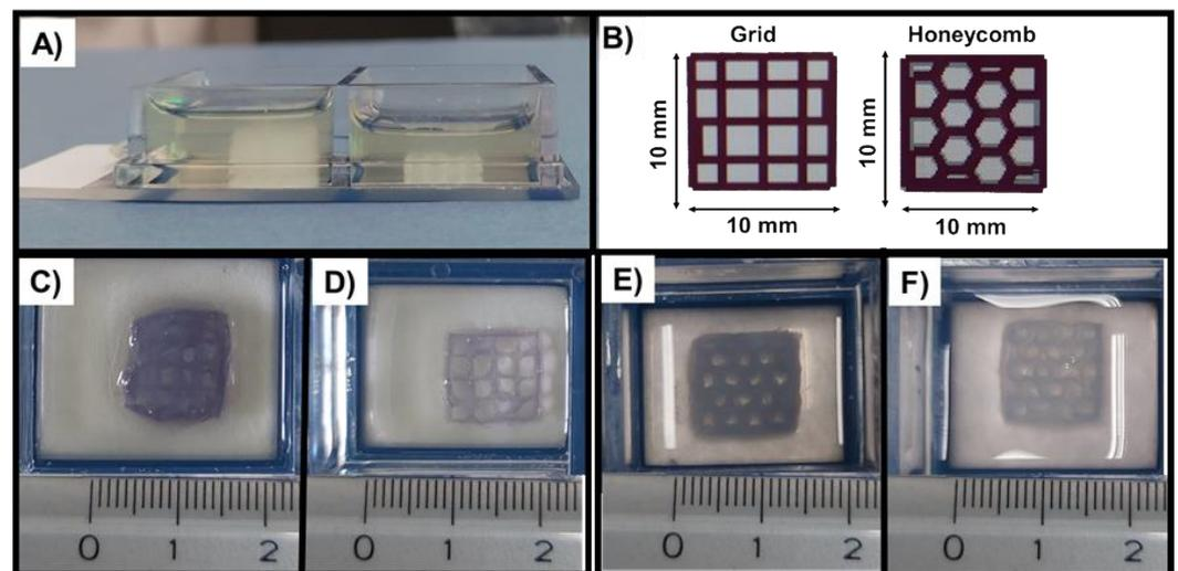
**Figure 9.** Images of 15 wt.% Alginate bath (A), scaffold design (B) and printed scaffolds after incubation at 37 °C for 24 h: GEN-Coll/MBG\_Sr4%, T1 and T2 (C,D, respectively) and GEN-Coll/nanoHA, T3 and T4 (E,F, respectively). Blue coloration of scaffolds is indicative of genipin crosslinking. Scaffold measurement 10 × 10 × 1 mm.
