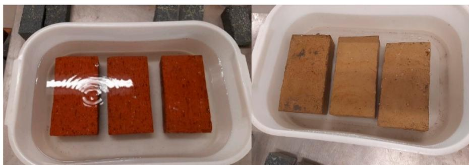
Figure 5. The wetting and drying cycle durability test setup for the clay and PW bricks.
