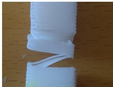
**Figure 4.** Macrographic image showing the loss of cohesion between the printed layers of the  $P_v$  specimen.
