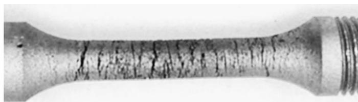
**Figure 11.** Smooth cylindrical specimen of a diameter of 5 mm after the combined action of tensile stress and hydrogen charging. Scale 1:2.
