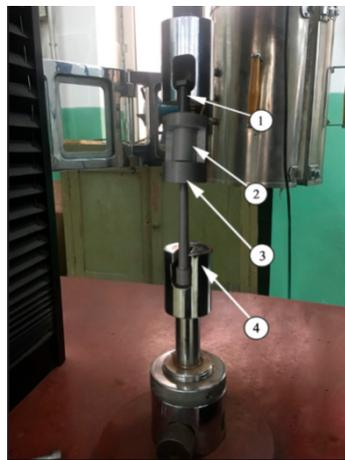
**Figure 3.** Tensile test device. 1—M12  $\times$  1.25 screw; 2—Magnesium alloy; 3—Special tooling; 4—Cupping machine.
