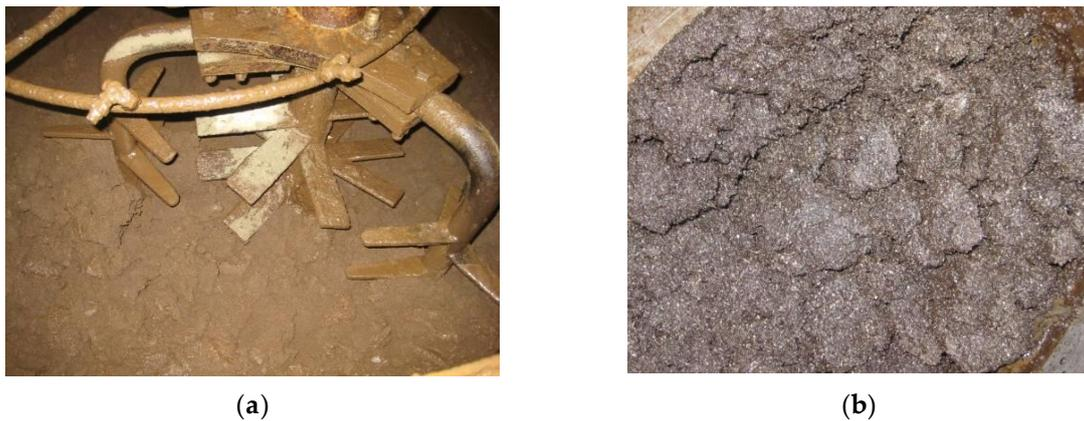
**Figure 1.** Flocculation and demulsification of emulsified asphalt in CAM I (a) Unable to mix, (b) Flocculation.
