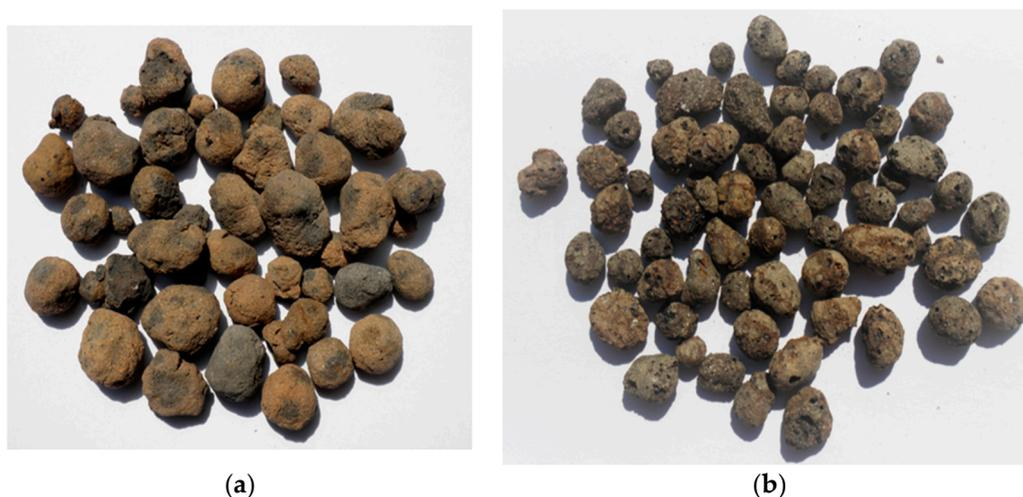
**Figure 1.** Lightweight aggregates used for concrete to be tested: (a) sintered fly ash and (b) expanded clay.
