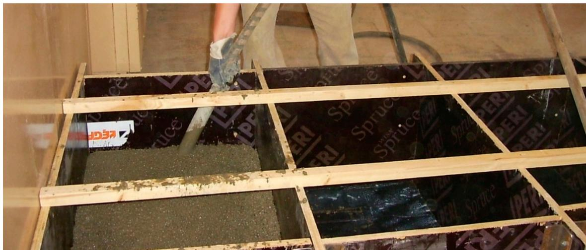
**Figure 2.** Preparation of concrete blocks for drilling cores.
