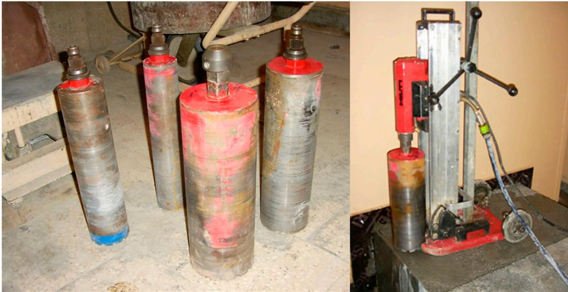
**Figure 3.** Types of drilling rigs used ( $d = 80, 100, 125, 150$  mm) and cutting out cores from a concrete block.
