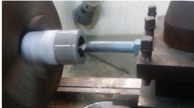
**Figure 3.** Wet drilling the binding samples using a lathing machine.
