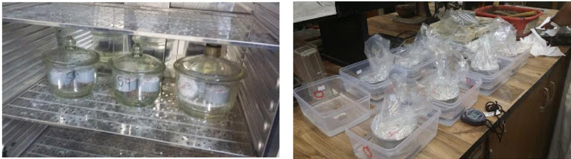
Figure 2. Sorptivity conditioning in KBr (left) and sorptivity testing setup (right).
