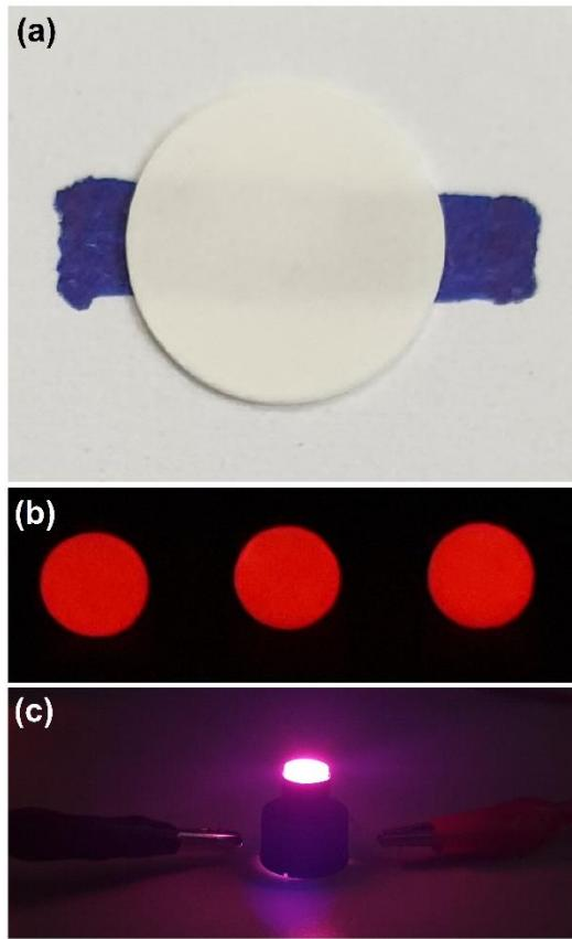
**Figure S3.** Digital images of: 0.73-mm-thick  $\text{Ba}_2\text{Y}_5\text{B}_5\text{O}_{17}:\text{Eu}^{3+}$  ceramic disk under daylight (a); 0.73, 0.98, and 1.20-mm-thick (from left to right)  $\text{Ba}_2\text{Y}_5\text{B}_5\text{O}_{17}:\text{Eu}^{3+}$  ceramic disks under 365 nm excitation (b); 1.20-mm-thick on top of 400 nm emitting LED (c).
