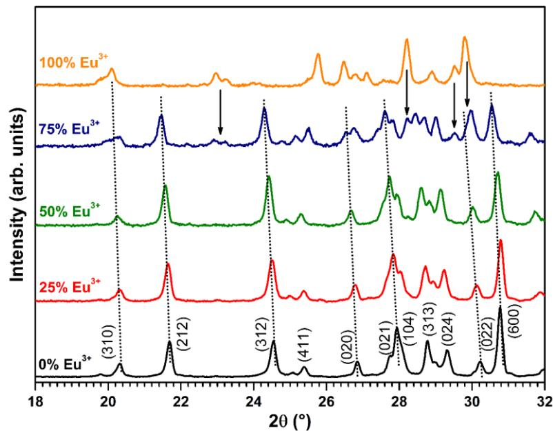
Figure S1. XRD patterns of  $\text{Ba}_2\text{Y}_5\text{B}_5\text{O}_{17}$ :  $\text{Eu}^{3+}$  phosphors.
