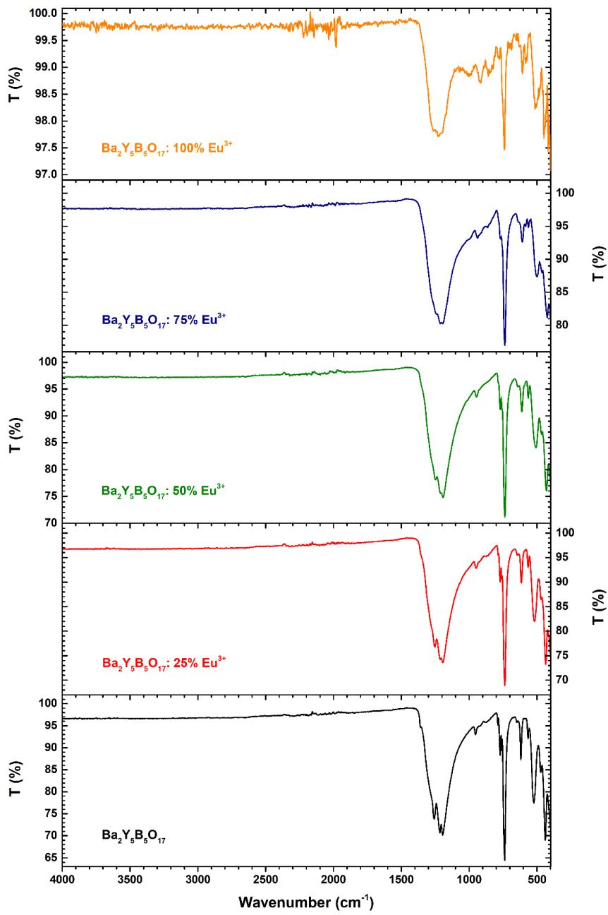
**Figure S2.** FTIR spectra of  $\text{Ba}_2\text{Y}_5\text{B}_5\text{O}_{17}$ :  $\text{Eu}^{3+}$  phosphors.
