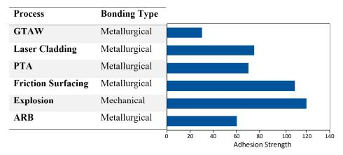
Figure 13. Bonding type and adhesion.
