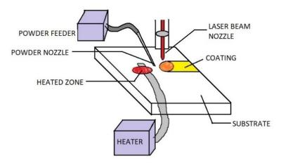
Figure 12. Pre-heating surface treatment.
