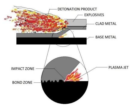
Figure 8. Explosion cladding.
