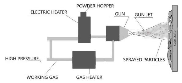
**Figure 3.** Cold spraying—a solid-state process.
