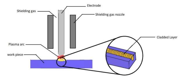
Figure 4. Schematics of gas tungsten arc welding (GTAW).
