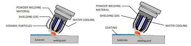
Figure 11. Synchronous Feeding (right) and Back Feeding (left) mechanisms.
