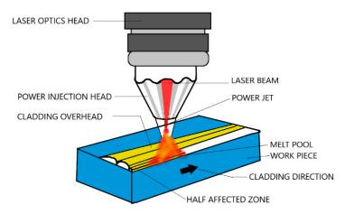
Figure 5. Laser cladding.
