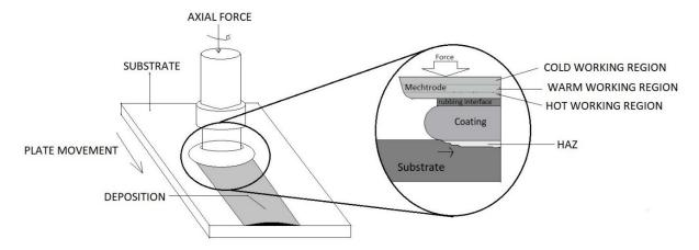
Figure 7. Schematics of friction surfacing.
