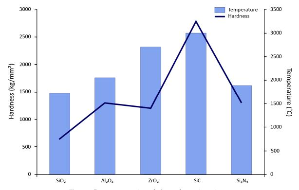
Figure 2. Property comparison of advanced ceramic coatings.
