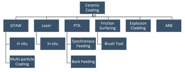
**Figure 10.** Processes and sub-systems for ceramic coating.
