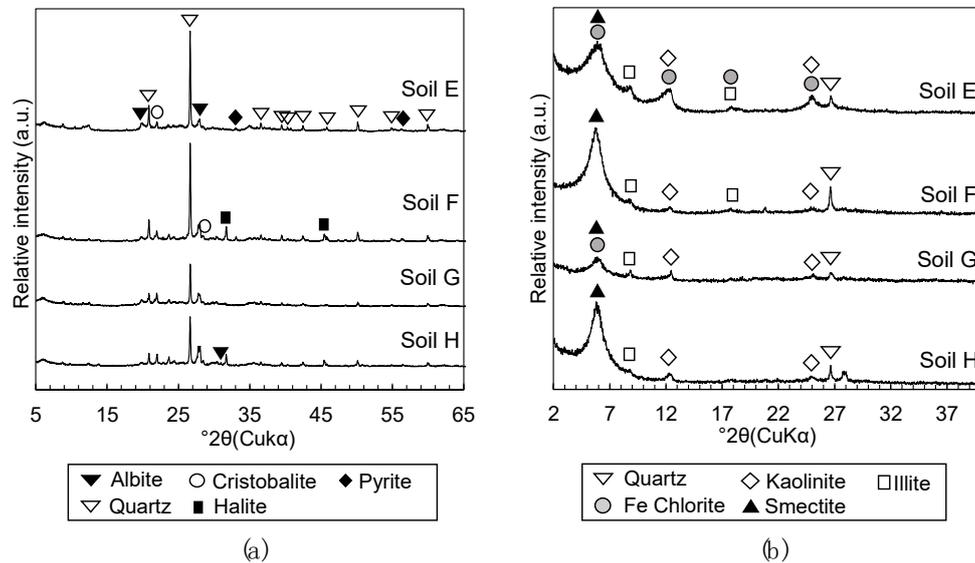
**Figure 1.** X-ray diffraction (XRD) patterns of (a) powdered dredged soil to detect bulk mineralogical phases and (b) oriented particles of dredged soils to detect clay mineralogical phases. Names of dredged soil samples are labeled on the upper right of each XRD pattern.
