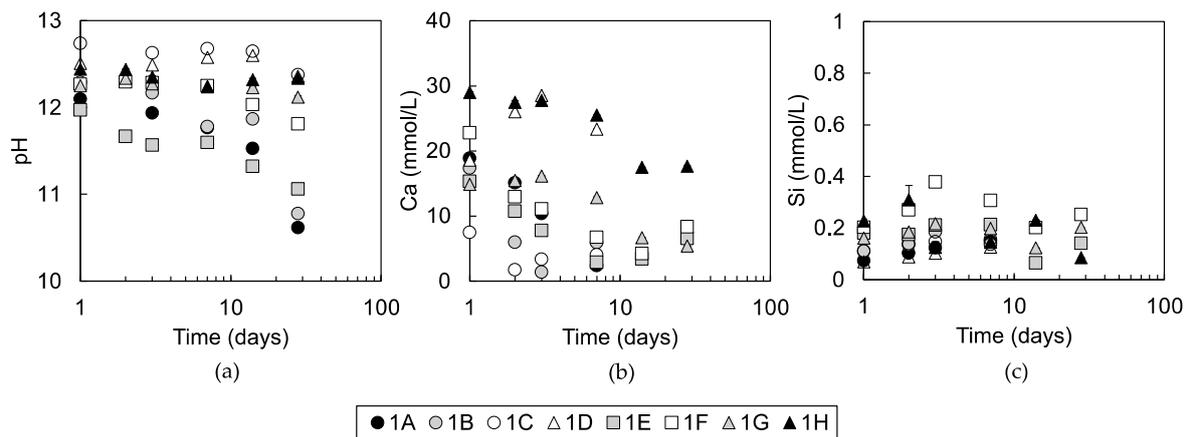
**Figure 8.** (a) pH of pore waters of mixtures 1A, 1B, 1C, 1D, 1E, 1F, 1G, and 1H at 1 to 28 days of curing, (b) calcium concentrations, and (c) silica concentrations of the pore waters of mixtures 1A, 1B, 1C, and 1D of 1 to 7 days of curing and of mixtures 1E, 1F, 1G, and 1H of 1 to 28 days of curing are plotted as a function of curing time. Standard errors of the measurements are plotted on the figures.
