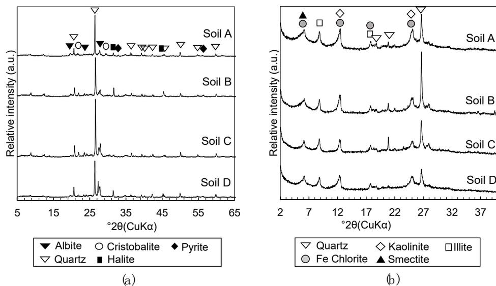
**Figure 2.** XRD patterns of (a) powdered dredged soil to detect bulk mineralogical phases and (b) oriented particles of dredged soils to detect clay mineralogical phases. Names of dredged soil samples are labeled on the upper right of each XRD pattern. From Toda et al. [13].
