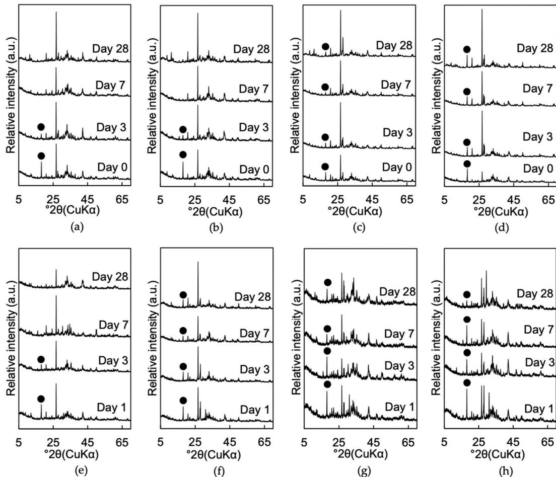
**Figure 7.** XRD patterns of (a) mixtures 1A, (b) 1B, (c) 1C, (d) 1D, (e) 1E, (f) 1F, (g) 1G, and (h) 1H cured for 1, 3, 7, and 28 days. XRD patterns (a–d) are from Toda et al. [13]. Black dot (●): Portlandite ( $\text{Ca}(\text{OH})_2$ ).
