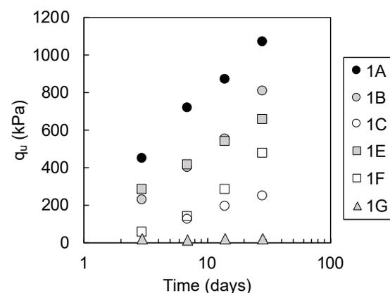
**Figure 6.** Unconfined compressive strength ( $q_u$ ) values of mixtures 1A, 1B, 1C, 1E, 1F, and 1G with curing time (data for mixtures 1A, 1B, and 1C are from Toda et al. [13]).
