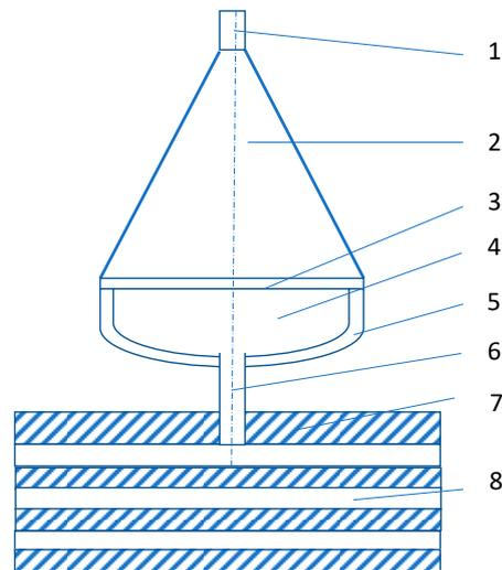
**Figure 2.** The impact of high-enthalpy plasma on the metal target: device diagram: 1—detonator; 2—explosive charge; 3—aluminum plate-piston; 4—working gas; 5—hemispherical copper compression chamber; 6—opening; 7—shield; 8—metal target.
