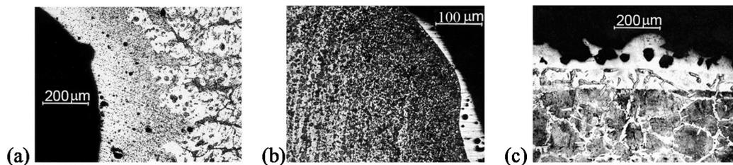
**Figure 3.** Microsection of metal surface layers after the impulse heating of the surface in contact with plasma from the explosive generator: (a) and (b)—the microstructure adjacent to the surface of the “piston” (a) and holder (b), respectively; (c)—the micro-section of the metal wall cut exposed to the plasma thermal shock.
