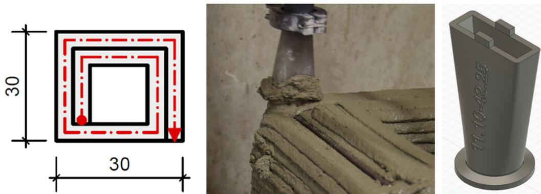
**Figure 2.** Sample geometriy (left), deposition of a layer on top of horizontal reinforcement (middle) and nozzle with tongue (right).
