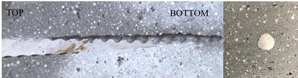
**Figure 15.** Void formation around the vertically inserted rebar (**left**). Bond between horizontally deposited rebar and mortar (**right**).
