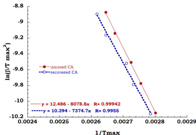
Figure 8. Comparison between Kissinger data obtained for the principal degradation stage.
