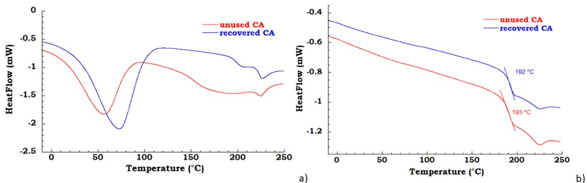
**Figure 2.** (a) differential scanning calorimetry (DSC) thermograms in the first heating scan of unused CA and recovered CA (b) DSC thermograms in the second heating scan of unused CA and recovered CA.
