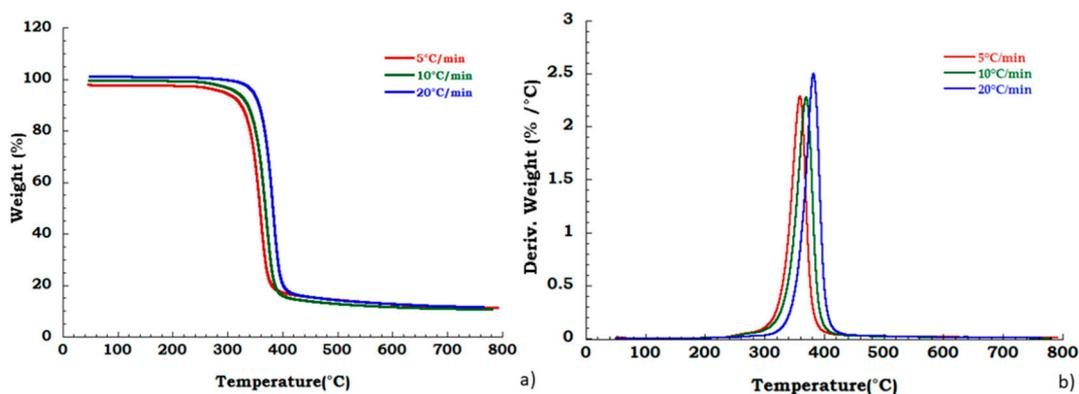
**Figure 5.** Thermogravimetric curves in nitrogen flow (a) TGA curves for recovered CA at different heating rate; (b) DTG curves for recovered CA at different heating rate.
