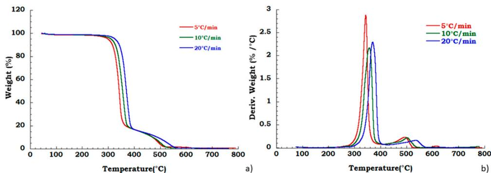
**Figure 7.** Thermogravimetric curves in air flow (a) TGA curves for recovered CA at different heating rate; (b) DTG curves for recovered CA at different heating rate.
