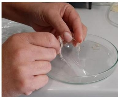
**Figure 12.** Transparent film of cellulose acetate recovered from cigarette butts.
