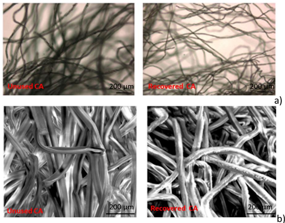
**Figure 1.** (a) Optical microscopy image (50×) of cellulose acetate fibers (CA) unused (left) and CA recovered (right); (b) SEM micrographs for CA unused (left) and CA recovered (right) at 800× magnification.
