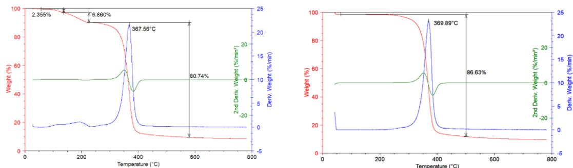
**Figure 3.** (a) TGA Thermograms on unused CA sample (10 °C/min, nitrogen flow); (b) TGA Thermograms on recovered CA sample (10 °C/min, nitrogen flow).
