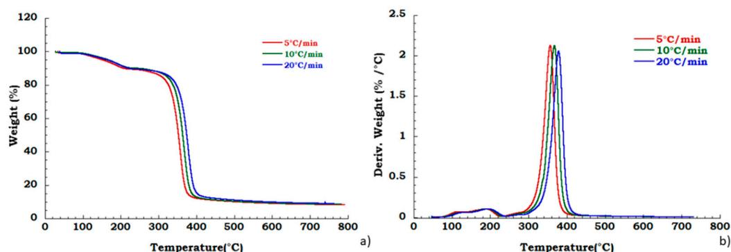
**Figure 4.** Thermogravimetric curves in nitrogen flow (a) unused CA at different heating rate; (b) DTG curves for unused CA.
