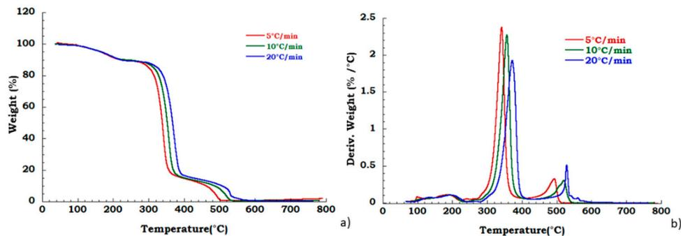
**Figure 6.** Thermogravimetric curves in air flow (a) unused CA at different heating rate; (b) DTG curves for unused CA.
