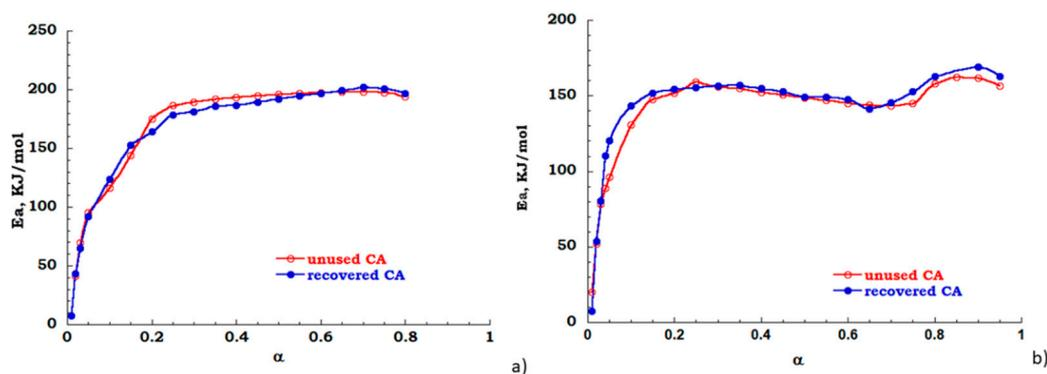
Figure 10. Energy profile derived from FOW (a) nitrogen flow; (b) air flow.
