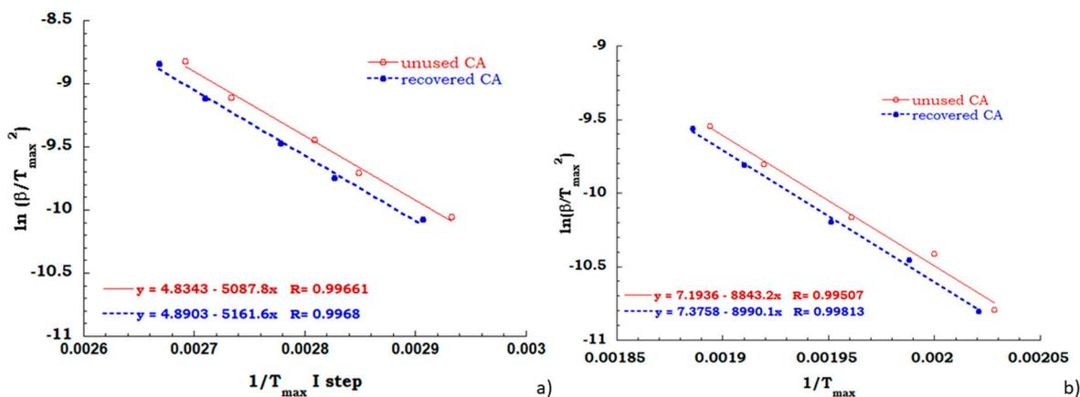
Figure 9. Kissinger data obtained for the deacetylation step (a) and charring stage (b) in air flow.
