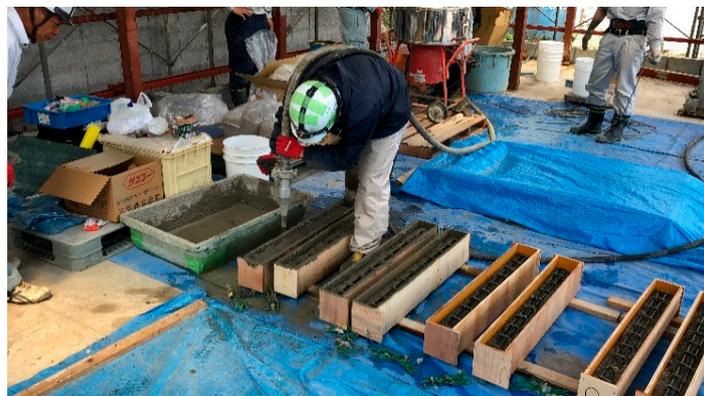
**Figure 3.** Spraying PCM on the removed section of RC beams.
