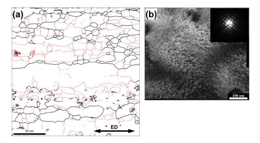
**Figure S3.** Initial microstructure of 6061 alloy: (**a**) EBSD grain-boundary map and (**b**) TEM image. ED is extrusion direction. In (**a**), low-and high-angle boundaries are depicted as red and black lines, respectively.
