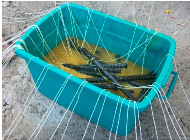
Figure 8. Cleaning with HCl solution.
