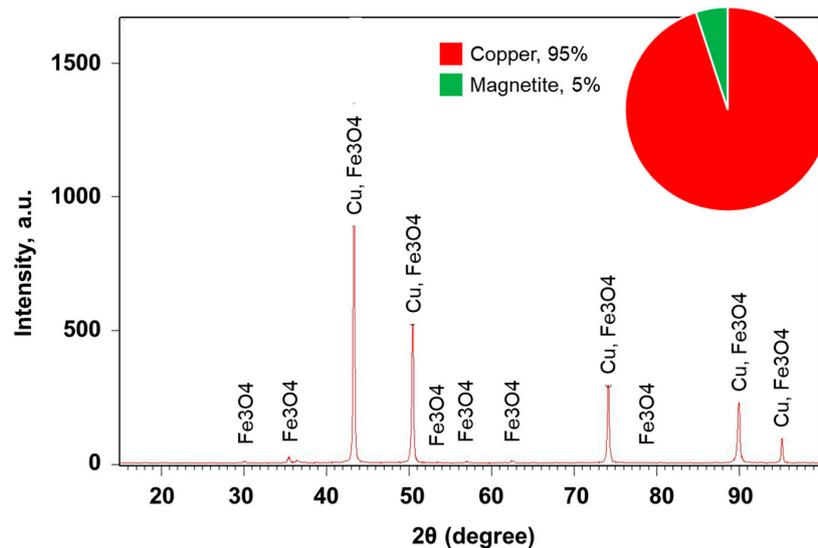
Figure 8. X-ray diffraction of Cu-5%Fe<sub>3</sub>O<sub>4</sub> nanocomposite sintered at 800 °C.
