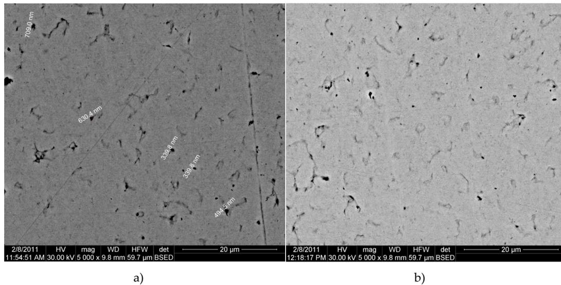
**Figure 14.** BSED microscopy images of Cu-15%Fe<sub>3</sub>O<sub>4</sub> nanocomposite obtained by sintering at 650 °C for 60 min (a) and 75 min (b).
