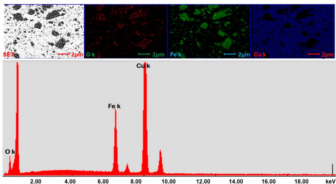
Figure 9. SEM images and EDS spectra recorded for a Cu-Fe<sub>3</sub>O<sub>4</sub> composite.
