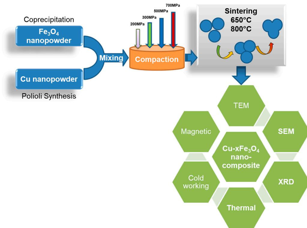
**Figure 1.** Illustration of the process diagram for synthesis and characterization of Cu-xFe<sub>3</sub>O<sub>4</sub> nanocomposites.
