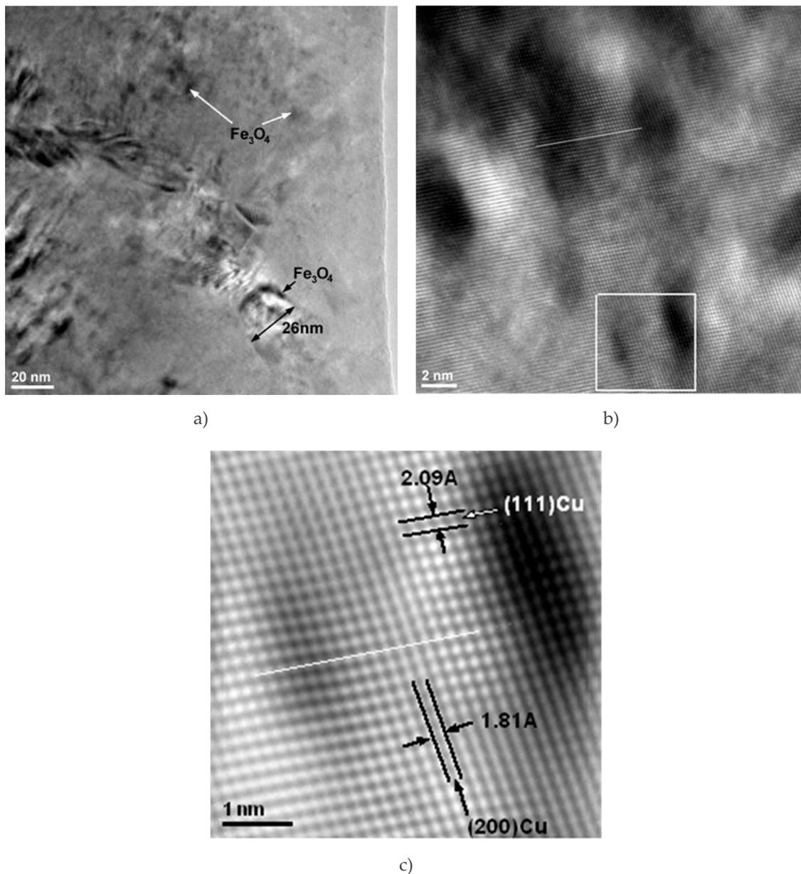
**Figure 11.** TEMBF images of the interface of Cu matrix and Fe<sub>3</sub>O<sub>4</sub> nanoparticle (a); image showing an agglomeration of magnetite nanometer particles embedded in the Cu crystallite matrix (b); inverse Fourier Transformation of the image shown in the white square marked in (b) at the bottom of the image (c).
