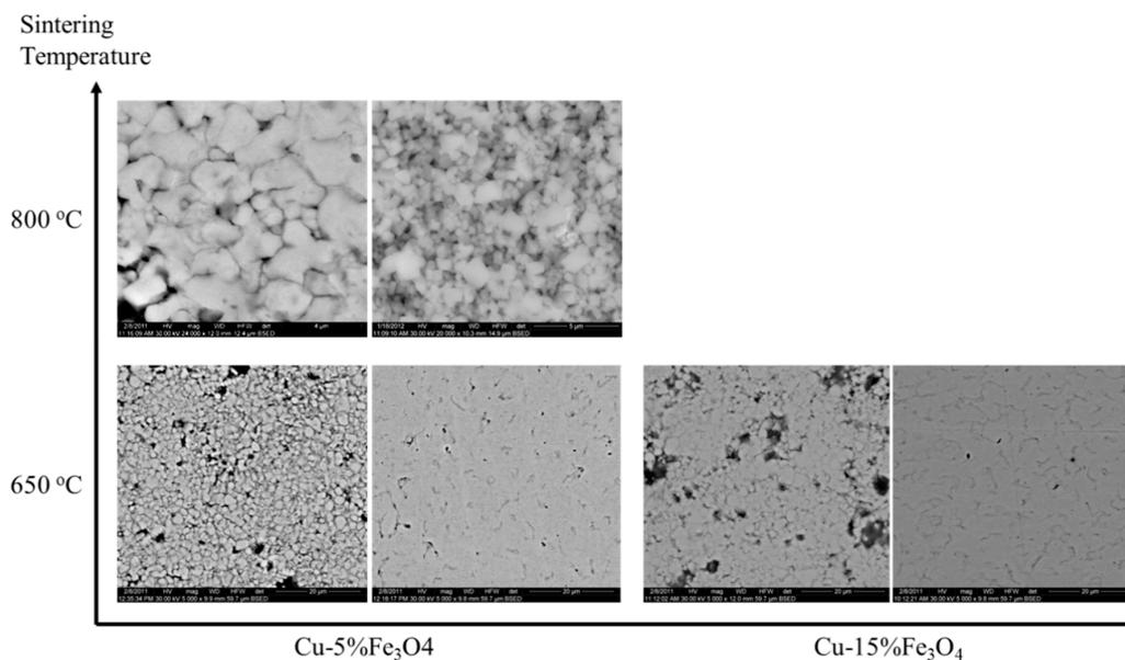
**Figure 12.** BSED microscopy images of Cu- $x\%$ Fe<sub>3</sub>O<sub>4</sub>, where  $x = 5$  and 15; each sintering condition has two images: before (left) and after (right) sintering.
