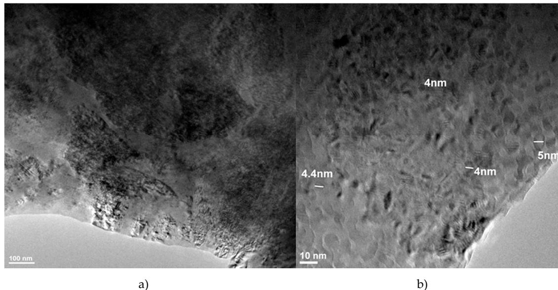
**Figure 10.** TEM images of Cu-15%Fe<sub>3</sub>O<sub>4</sub> sintered at 800 °C showing the distribution (a) and an agglomeration of Fe<sub>3</sub>O<sub>4</sub> nanoparticles embedded into the Cu matrix (b).
