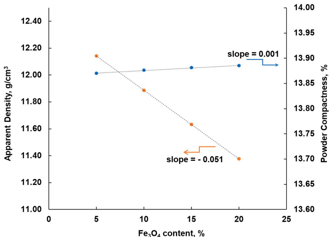
**Figure 3.** Variation of apparent density and powder compactness with the  $Fe_3O_4$  content in the powder blend.
