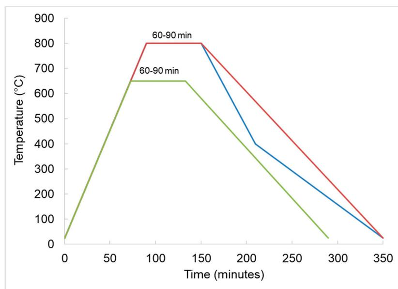
Figure 7. Sintering heating schedule for  $\text{Cu-xFe}_3\text{O}_4$ .
