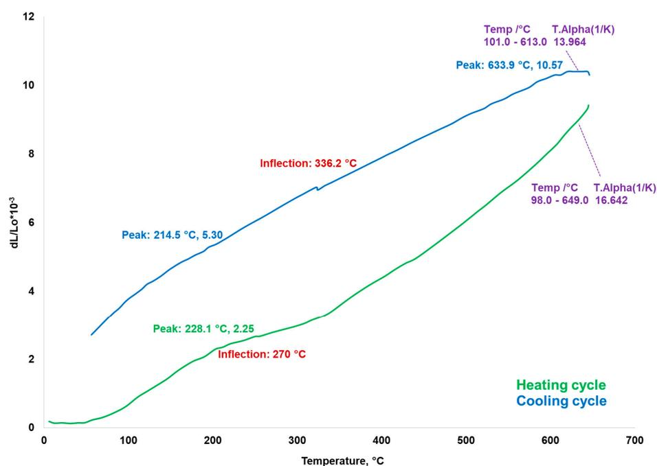
Figure 18. Shrinkage profile as a function of temperature for Cu-5%Fe<sub>3</sub>O<sub>4</sub> sample.
