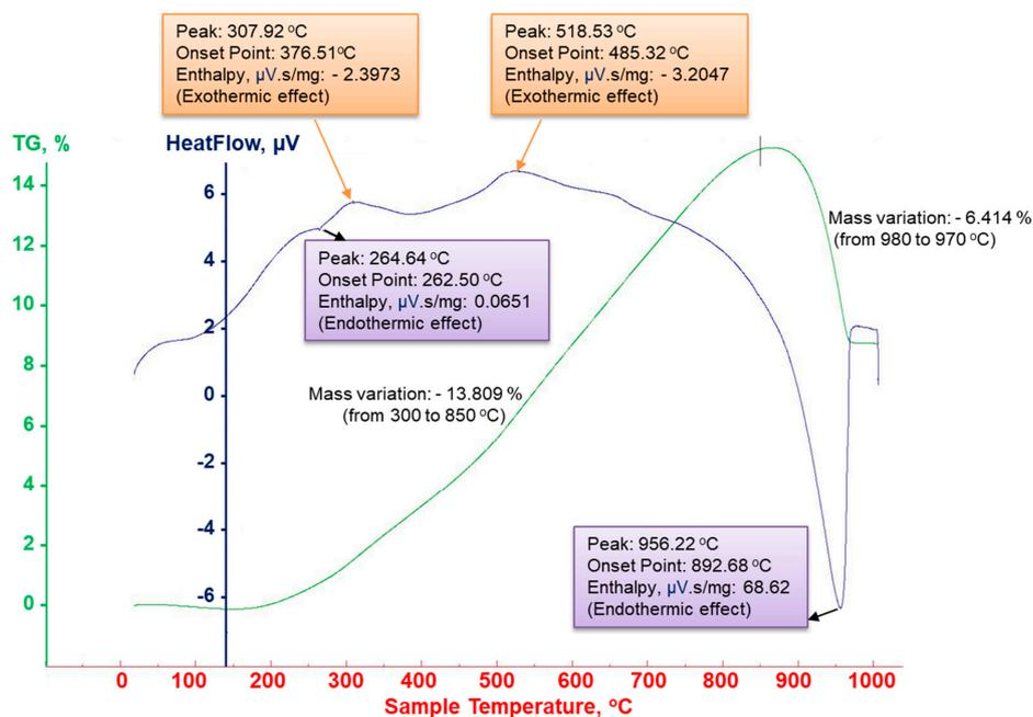
**Figure 17.** DSC-TG thermogram of Cu-Fe<sub>3</sub>O<sub>4</sub> nanocomposite.
