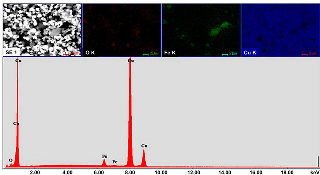
**Figure 2.** SEM image and the associated elemental mappings of Cu, O and Fe, along with the EDS spectra for a powder mixture of Cu-15%Fe<sub>3</sub>O<sub>4</sub> (line bar is 2 μm).
