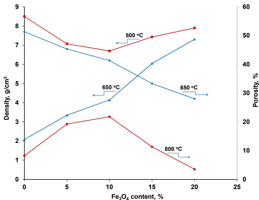
**Figure 13.** Variation of the density and porosity of composites as a function of the Fe<sub>3</sub>O<sub>4</sub> content.
