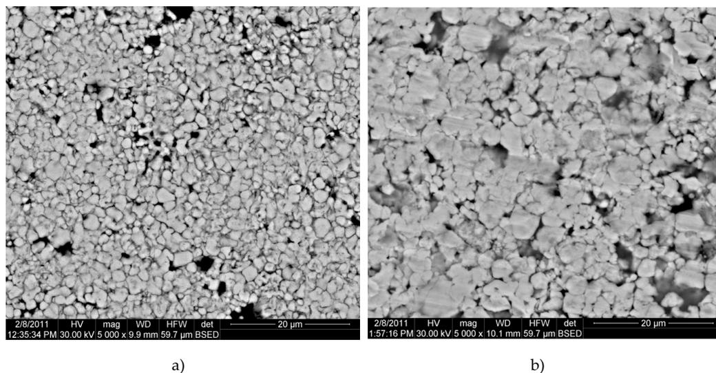
**Figure 5.** BSED microscopy images of the  $\text{Cu-15\%Fe}_3\text{O}_4$  samples compacted at 500 MPa (a) and 700 MPa (b).
