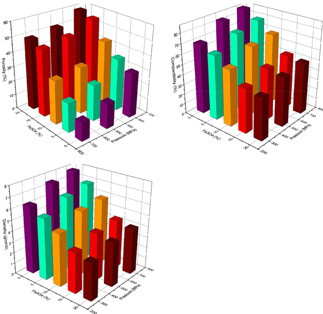
**Figure 6.** 3-D chart representation of the powder porosity, compressibility and density as a function of the Fe<sub>3</sub>O<sub>4</sub> amount and compacting pressure.
