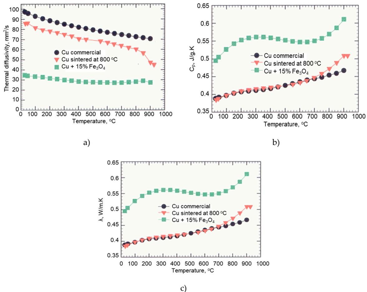
**Figure 16.** Thermal properties of commercial Cu, nanocomposites of Cu and Cu-15%Fe<sub>3</sub>O<sub>4</sub> sintered at 800 °C: (a) thermal diffusivity; (b) specific heat; and (c) thermal conductivity.
