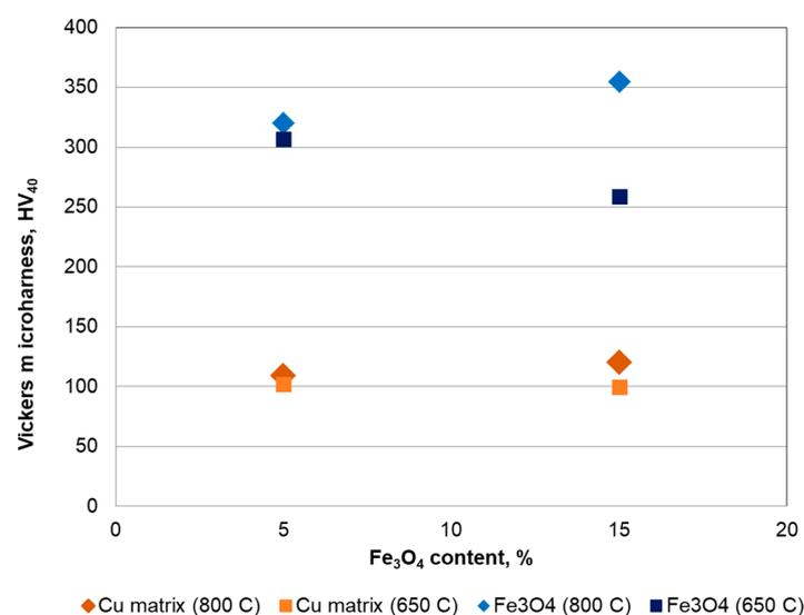
**Figure 21.** Vickers microhardness (averaged values) of  $\text{Cu-5\%Fe}_3\text{O}_4$  sintered at  $650$  and  $800\text{ }^\circ\text{C}$ .
