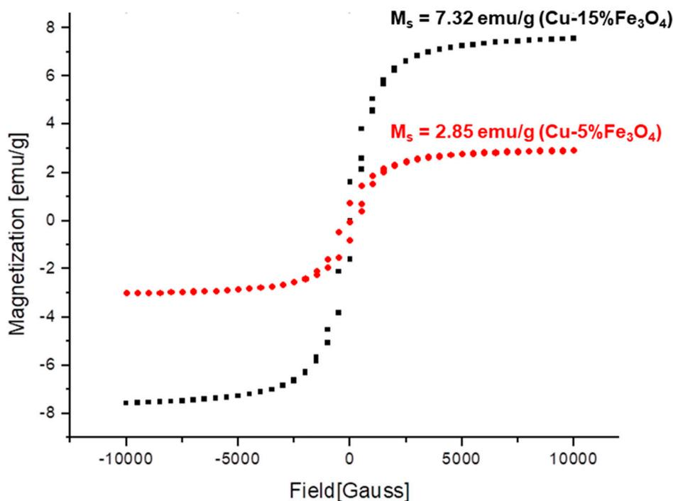
**Figure 22.** Magnetization curves of Cu-5%Fe<sub>3</sub>O<sub>4</sub> and 15%Fe<sub>3</sub>O<sub>4</sub> nanocomposites performed at room temperature.
