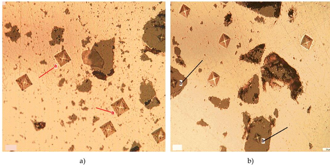
**Figure 20.** Optical images of the Vickers microhardness measurements on Cu matrix (a) and on  $\text{Fe}_3\text{O}_4$  particle agglomeration (b).
