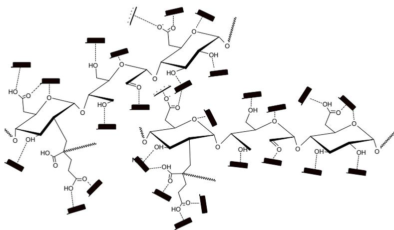
Figure S3. Schematic representation of the interactions between bentonite and S-g-IA\_APS.
