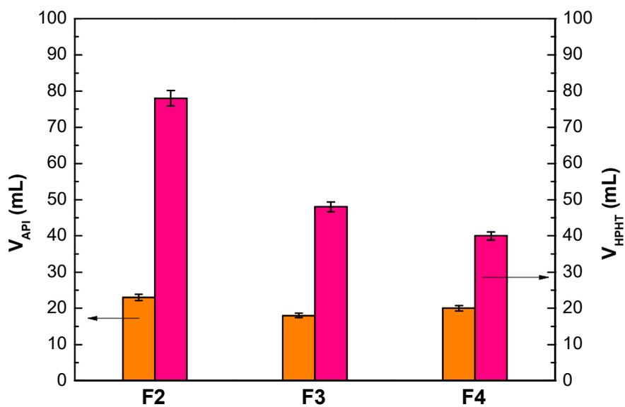
Figure S4. Comparison between  $V_{API}$  and  $V_{HPHT}$  of drilling fluids.
