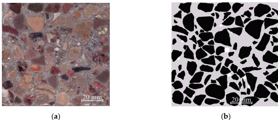
**Figure 6.** View of the concrete sample CW0, (a) scanned; (b) analyzed by employing computer graphic software: a white color is used to indicate pores; light gray—newly created cement stone with fine aggregate; black—coarse aggregates.
