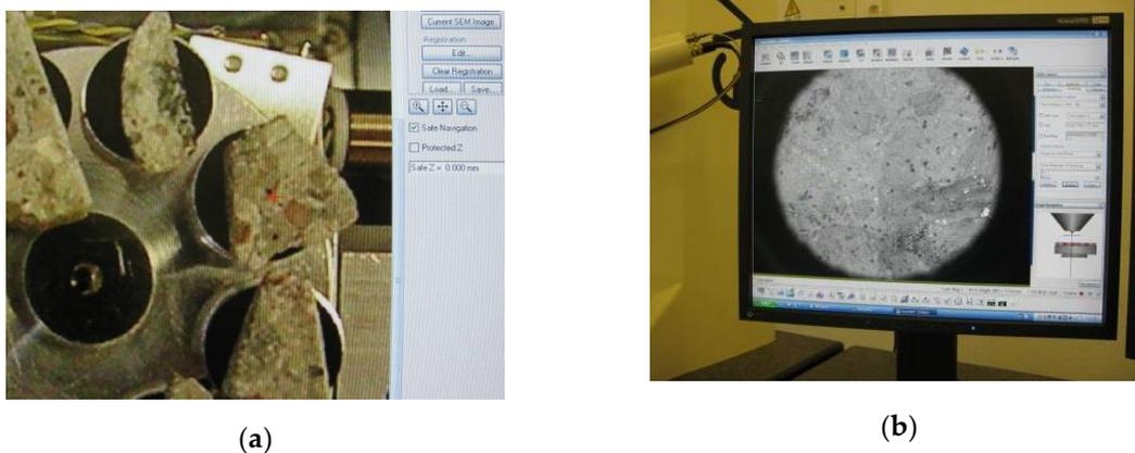
Figure 4. View of SEM search system: (a) real view of samples: (b) view of sample placed in the microscope.
