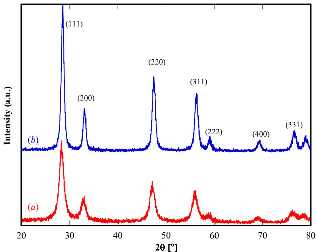
Figure 2. XRD patterns of as-synthesized (red) and calcined (blue) SPDC-NH<sub>3</sub>.
