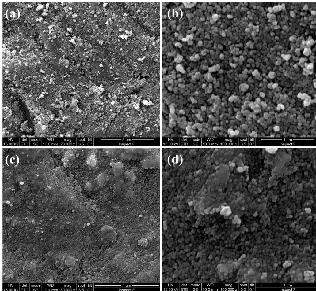
**Figure 9.** SEM micrographs of sintered SPDC-NH<sub>3</sub> at 50 V/cm and 20 mA/mm<sup>2</sup> (a,b) and 40 mA/mm<sup>2</sup> (c,d).
