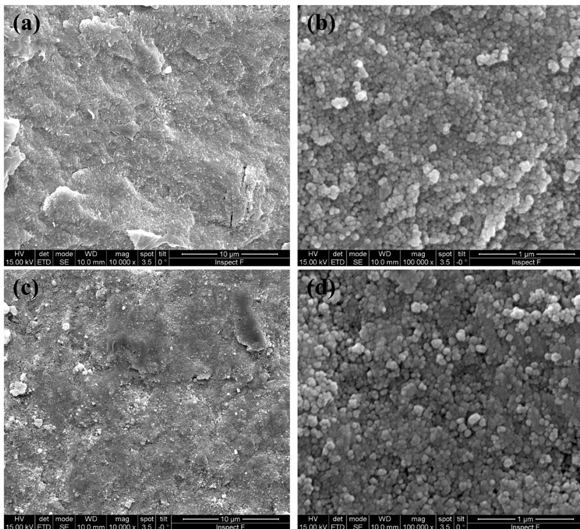
**Figure 7.** SEM micrographs of sintered SPDC-AC with ramp cycle; ramp up to 12 mA/mm<sup>2</sup> (a,b) and ramp up to 18 mA/mm<sup>2</sup> (c,d).
