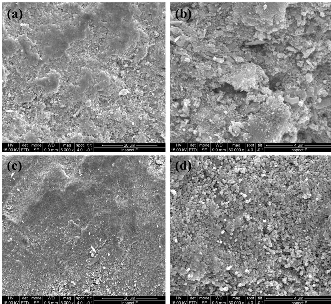
**Figure 5.** SEM micrographs of flash-sintered SPDC-AC (a,b) and GPDC-AC (c,d) samples under a current limit of 20 mA/mm<sup>2</sup>.
