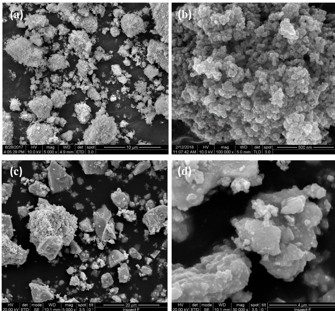
**Figure 3.** SEM micrographs of calcined SPDC-AC (a,b) and SPDC-NH<sub>3</sub> (c,d) powders.
