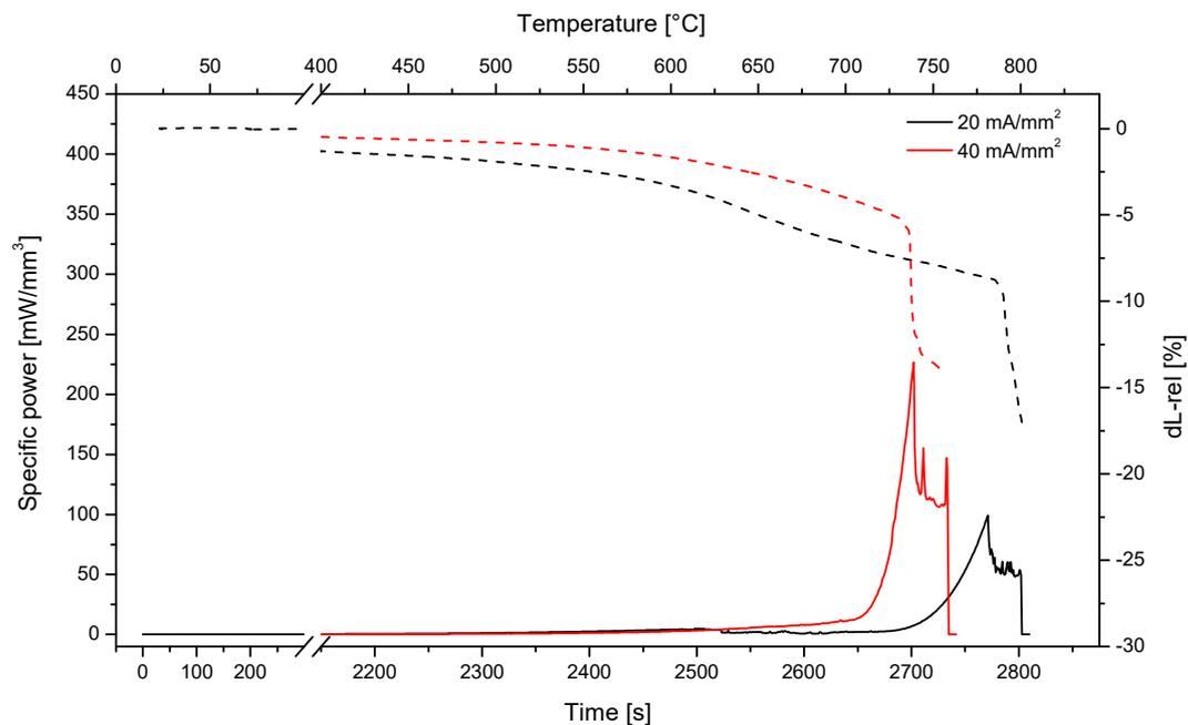
**Figure 8.** Specific power density and dilatometric plot for SPDC-NH<sub>3</sub> samples treated using 50 V/cm and different current limits.
