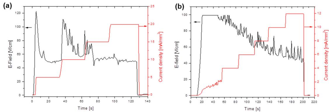
**Figure 6.** Electrical data for the two current ramps adopted in this work: up to 20 mA/mm<sup>2</sup> (a) and 12 mA/mm<sup>2</sup> (b).
