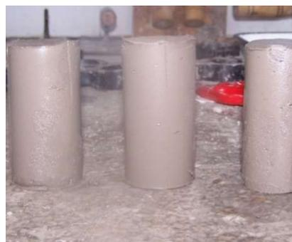
**Figure 2.** Sample after demolding.
