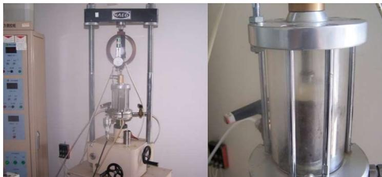
Figure 3. Unconfined compressive strength test by triaxial shear tester.
