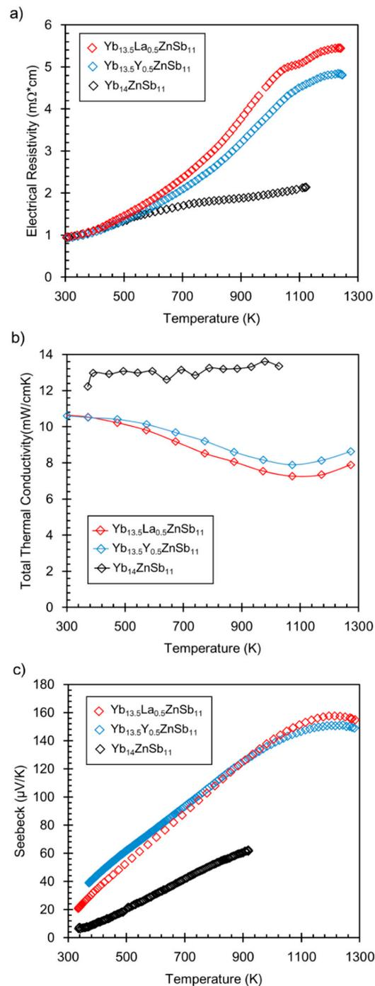
**Figure 4.** (a) Electrical resistivity, (b) thermal conductivity, and (c) Seebeck for the  $\text{Yb}_{13.5}\text{RE}_{0.5}\text{ZnSb}_{11}$  (RE = Y, La) compounds plotted against those of  $\text{Yb}_{14}\text{ZnSb}_{11}$  ( $\text{Yb}_{14}\text{ZnSb}_{11}$  data from the work of [9]).
