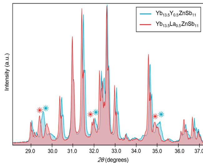
**Figure 3.** Powder X-ray diffraction (PXRD) patterns of  $\text{Yb}_{13.5}\text{Y}_{0.5}\text{ZnSb}_{11}$  (filled in blue) and  $\text{Yb}_{13.5}\text{La}_{0.5}\text{ZnSb}_{11}$  (filled in red) from  $28^\circ$  to  $37^\circ$   $2\theta$ . Unidentified peaks in each pattern are marked by asterisks in respective colors.
