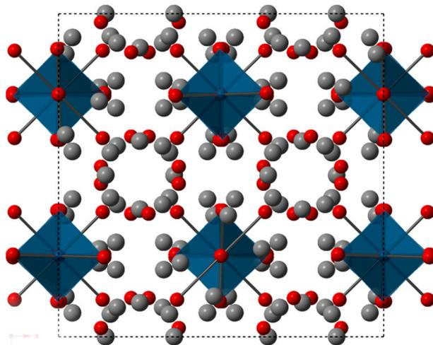
**Figure 1.** A view of the structure of  $\text{Yb}_{14}\text{ZnSb}_{11}$  down the  $c$  axis. Yb atoms are grey, Sb atoms are in red, and the blue tetrahedra are the  $\text{ZnSb}_4$  units.
