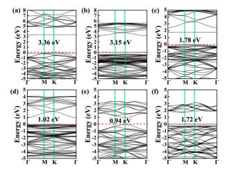
**Figure 5.** Band structures of CH<sub>2</sub>O on the surface of the (**a**) BN, (**b**) AlN, (**c**) GaN, (**d**) InN, (**e**) BP, and (**f**) P monolayers.
