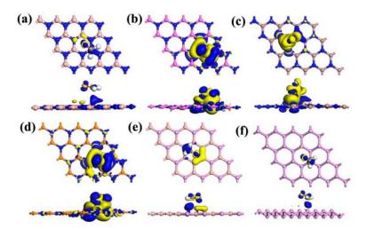
**Figure 3.** Charge density differences for the  $CH_2O$  adsorbed on the surface of the (a) BN, (b) AlN, (c) GaN, (d) InN, (e) BP, and (f) P monolayers with an isosurface value of  $0.003 \text{ e}/\text{Å}^3$ . The blue and yellow contours denote the increase and decrease of electrons, respectively.
