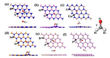
**Figure 2.** Most stable adsorption structures of  $CH_2O$  on the surface of the (**a**) BN, (**b**) AlN, (**c**) GaN, (**d**) InN, (**e**) BP, and (**f**) P monolayers.
