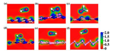
**Figure 6.** Slices of charge densities for the  $CH_2O$  adsorbed on the (a) BN, (b) AlN, (c) GaN, (d) InN, (e) BP, and (f) P monolayers. The charge density ranges from 0 to 2 e/A<sup>3</sup>.
