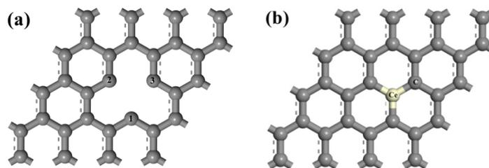
Figure 1. Physical models of graphene: (a) VG; (b) Ce-doped graphene.
