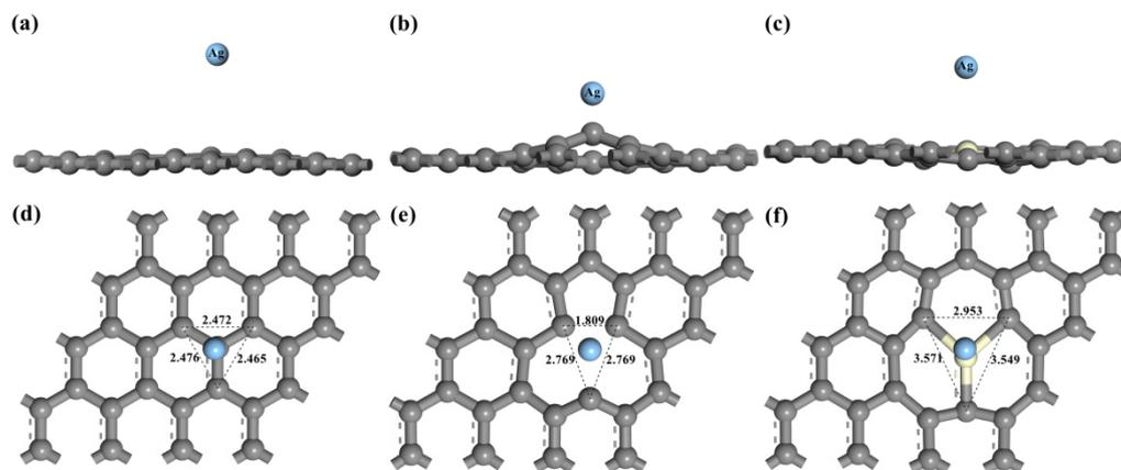
**Figure 2.** Geometric structures of graphene with the adsorbed Ag atom: (a) front view of intrinsic graphene; (b) front view of VG; (c) front view of Ce-doped graphene; (d) top view of intrinsic graphene; (e) top view of VG; (f) top view of Ce-doped graphene.
