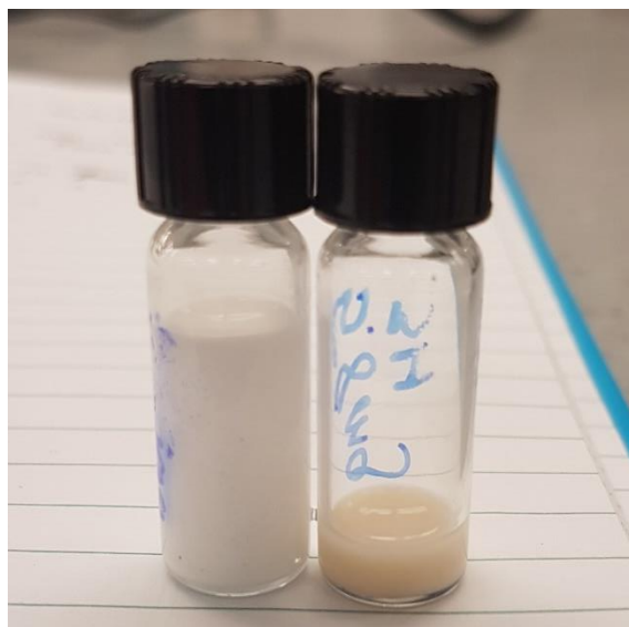
Figure S8. Comparison of pure white commercial ZnO (left) and 2-h synthesized sample (right) in ethanol depicting the off-white color obtained for the synthesized samples.
