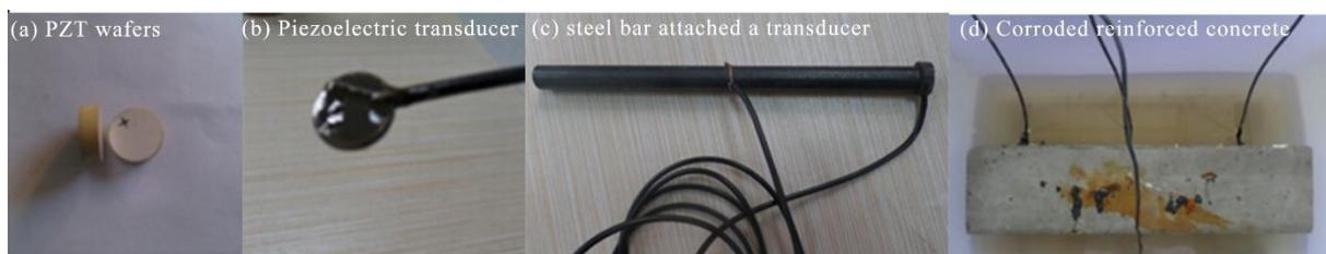
**Figure 2.** Photographs of the piezoelectric transducer and corroded reinforced concrete. (a) PZT (Lead Zirconate Titanate) wafers; (b) Piezoelectric transducers; (c) Steel bar attached a transducer; (d) Corroded reinforced concrete.
