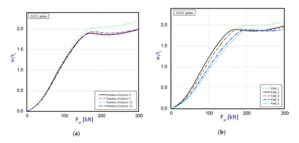
**Figure 6.** Static load vs. the normalized deflection (FEM) in the middle of the plate for the plate CCCC: (a) a different number of layers (b) different variants.
