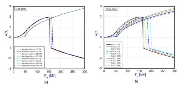
**Figure 5.** Static load vs. the normalized deflection in the middle of the plate for the plate SCSC: (**a**) a different number of layers (**b**) different variants.
