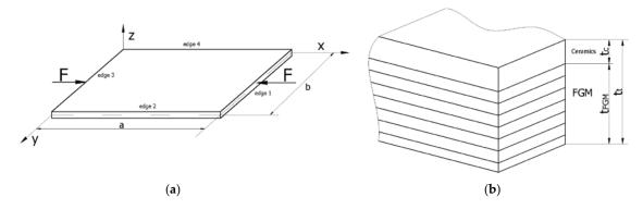
**Figure 1.** A functionally graded material (FGM) plate with its dimensions and a coordinate system (**a**) and a schematic view of the material distribution (**b**).
