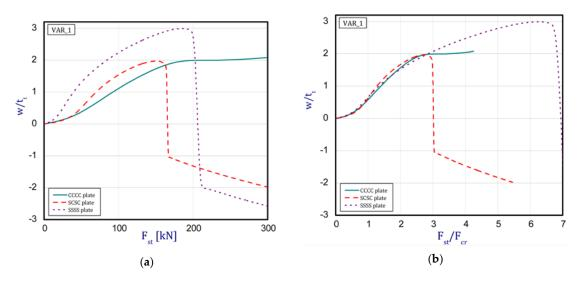
**Figure 7.** Comparison of the plots (FEM) for Var\_1: (**a**) static load vs. the normalized deflection and (**b**) the critical load of static load vs. the normalized deflection.
