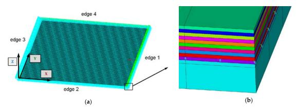
Figure 3. Discrete model with boundary conditions (a) and a view of the plate corner (b).
