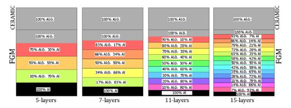
Figure 2. Material distribution versus a number of layers.
