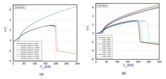
**Figure 4.** Static load vs. the normalized deflection in the middle of the plate for the plate SSSS: (**a**) a different number of layers (**b**) different variants.
