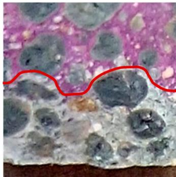
Figure 4. Deeper carbonation front in porous LWA than in matrix [86].
