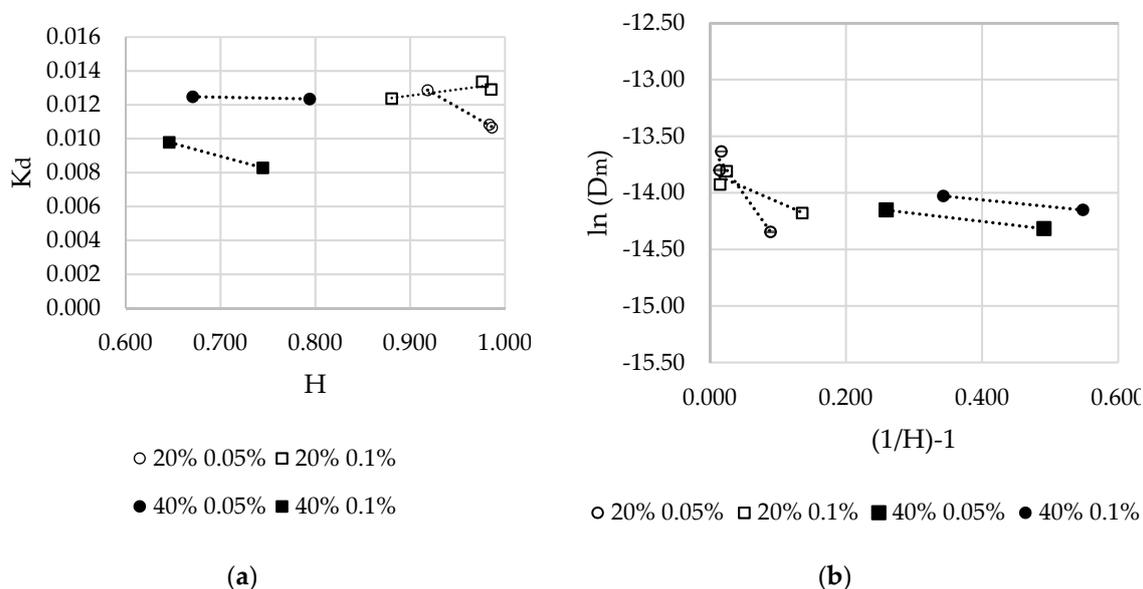
**Figure 5.** (a) Partition coefficients of Rhodamine B in PEGDA 575-2000 formulations according to hydration; (b) logarithm of diffusion coefficients of Rhodamine B in PEGDA575-2000 formulations as a function of inverse hydration.
