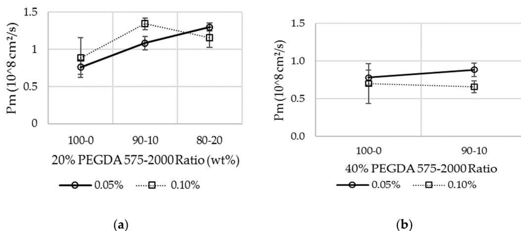
**Figure 3.** Permeation coefficients of (a) 20% and (b) 40% PEGDA formulations.
