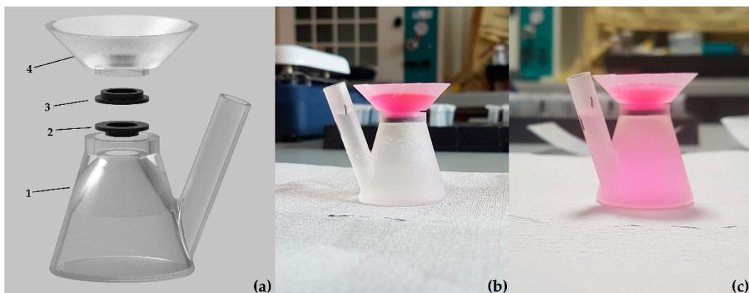
**Figure 1.** (a) Component parts of vertical transwell system, 3D-printed using Formlabs clear (1,4) and flexible (2,3) materials, wherein a Mixed-Molecular-Weight Poly(ethylene) Glycol Diacrylate (PEGDA) disc is placed between parts 2 and 3. Friction fit between parts 1 and 4 ensures that the system remains together; (b) transwell system at  $t = 0$  h; (c) transwell system at  $t = 12$  h.
