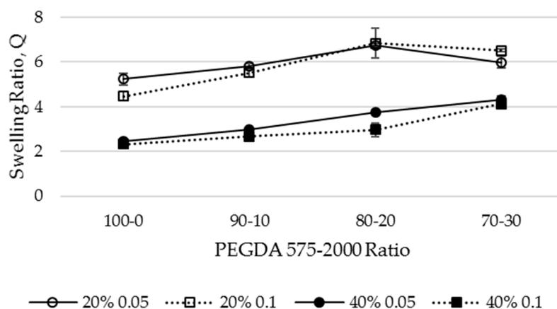
Figure 2. Difference in swelling ratio (Q) for various PEGDA575-2000 formulations.
