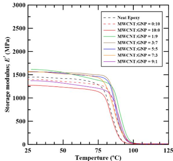
**Figure 5.** Temperature dependence of the storage modulus  $E'$  of the epoxy composites with various MWCNT:GNP ratios.
