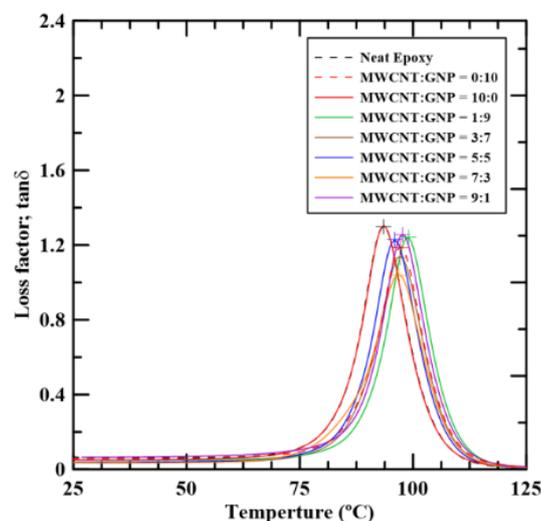
**Figure 6.** Temperature dependence of the loss factor  $\tan \delta$  of the epoxy composites with various MWCNT:GNP ratios.
