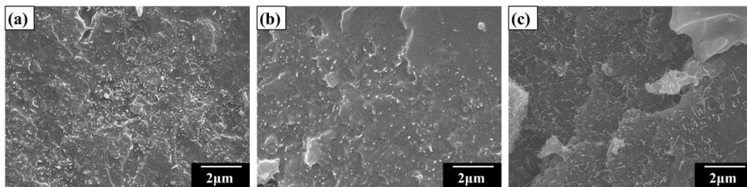
**Figure 4.** SEM images of the epoxy composites with the MWCNT:GNP ratios of (a) 10:0, (b) 5:5, and (c) 7:3 obtained after the SDS treatments.
