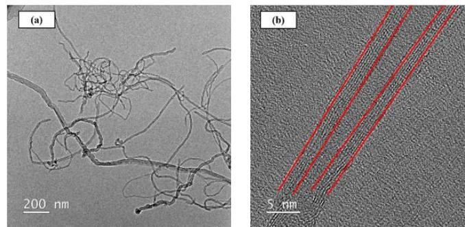
**Figure 1.** TEM images of as-received MWCNTs: (a)  $\times 200$ , (b)  $\times 10$  k.
