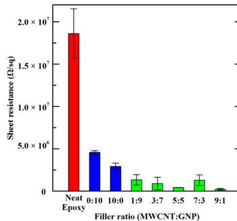
**Figure 8.** Variation of measured sheet resistances of the studied nanocomposites with the employed filler ratios in the specimen preparation.
