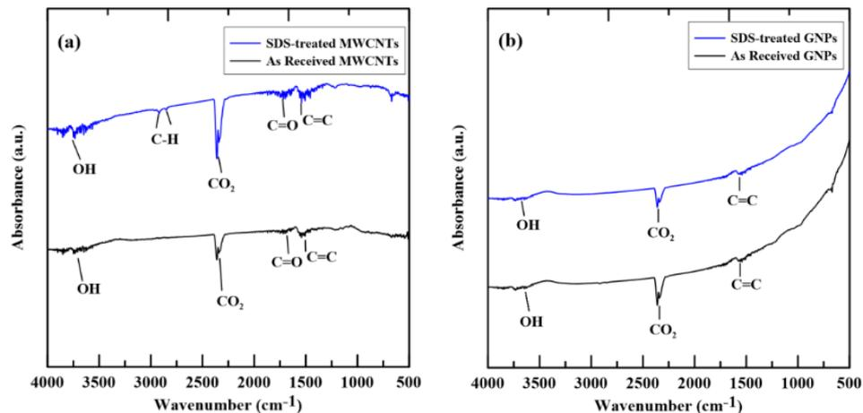
**Figure 3.** Comparison of the FT-IR spectra between the as-received and SDS treated carbon nano-fillers: (a) MWCNTs and (b) GNPs.
