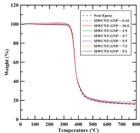
**Figure 9.** Relationship between the weight loss of the epoxy composites with various MWCNT:GNP ratios and temperatures obtained using TGA analysis.
