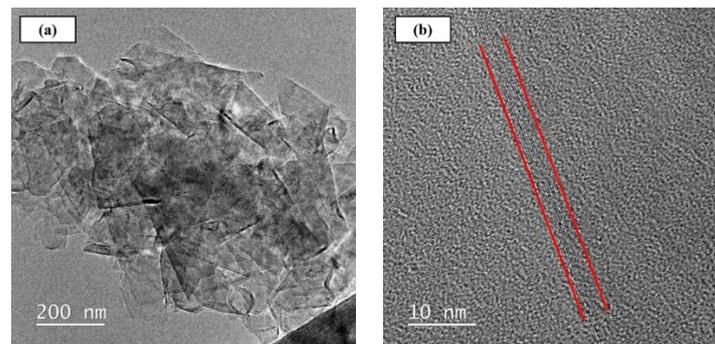
**Figure 2.** TEM images of as-received GNPs: (a)  $\times 200$ , (b)  $\times 10$  k.
