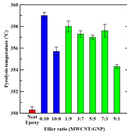
**Figure 10.** Variation of measured pyrolysis temperatures of the studied nanocomposites  $T_d$  with the employed filler ratios in the specimen preparation.
