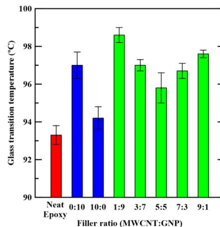
**Figure 7.** Variation of measured glass transition temperatures of the studied nanocomposites  $T_g$  with the employed filler ratios in the specimen preparation.
