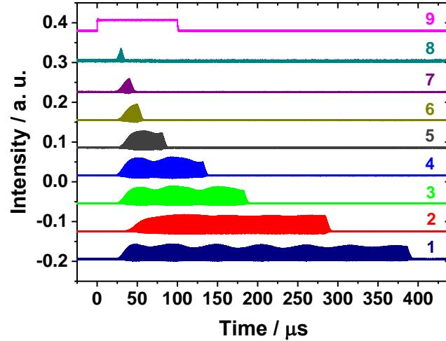
**Figure S3.** Macropulses of THz radiation with wavenumber of  $239\text{ cm}^{-1}$ . Pulse durations are (1) 400  $\mu\text{s}$ ; (2) 300  $\mu\text{s}$ ; (3) 200  $\mu\text{s}$ ; (4) 150  $\mu\text{s}$ ; (5) 100  $\mu\text{s}$ ; (6) 70  $\mu\text{s}$ ; (7) 60  $\mu\text{s}$ ; (8) 50  $\mu\text{s}$  (multiplied by 5); (9) trigger signal. Each subsequent pulse is vertically shifted.
