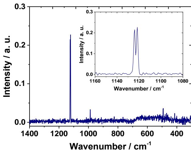
**Figure S8.** Spectrum of radiation used in the experiments at the third FEL of the NovoFEL facility. Inset shows closer view of the spectrum.
