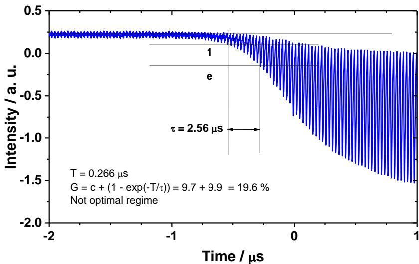
**Figure S14.** Gain calculation for the third FEL. Characteristic exponential time is 2.56  $\mu$ s.
