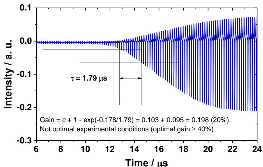
**Figure S10.** Gain calculation for the first FEL. Characteristic exponential time is 1.79  $\mu\text{s}$ .
