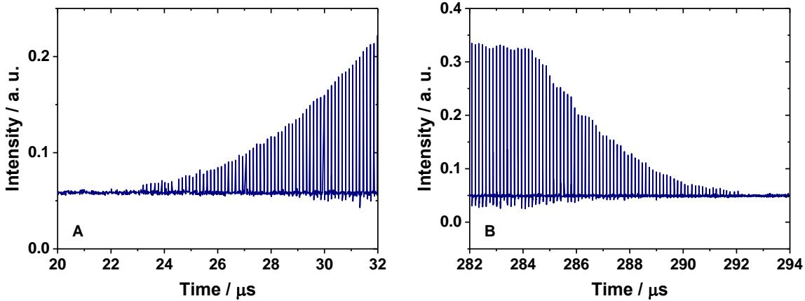
**Figure S4.** (A) The rising edge of the macropulse with 300  $\mu\text{s}$  duration; (B) The falling edge of another macropulse with 300  $\mu\text{s}$  duration. The individual pulses of THz radiation with the frequency of 7.5 MHz are clearly visible.
