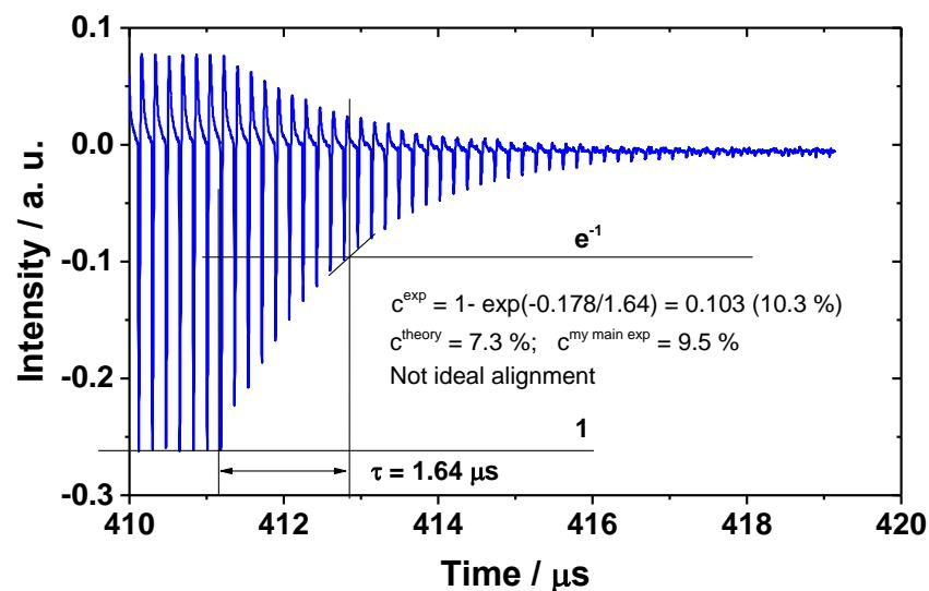
**Figure S9.** Calculation of losses for the first FEL. Characteristic exponential time is  $1.64 \mu\text{s}$ .
