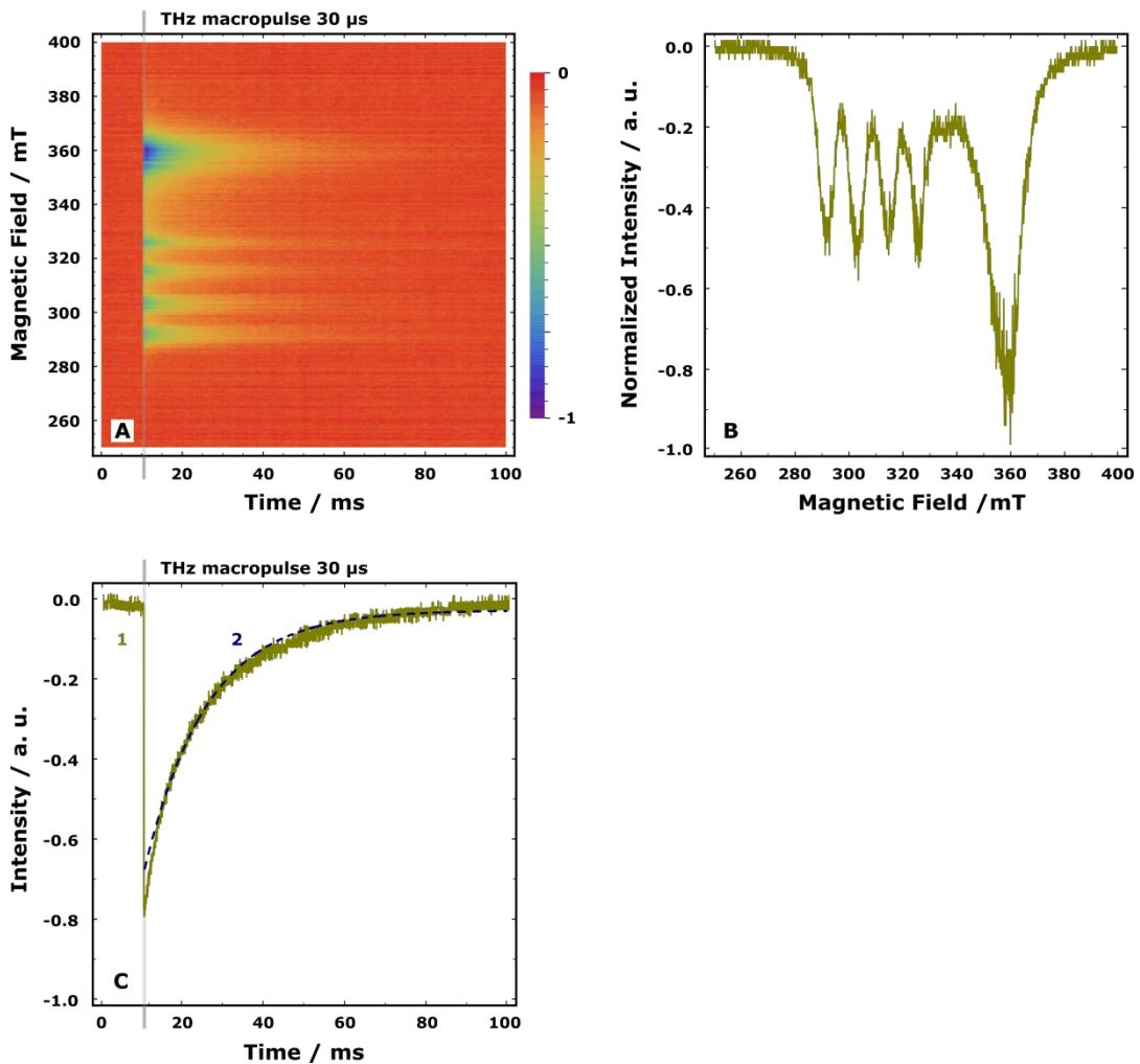
**Figure S15.** (A) Normalized TR EPR spectrum of  $\text{Cu}(\text{hfac})_2\text{LPr}$  (see Figures 5 and S16 for the structure) measured at 7 K using THz macropulses of 30  $\mu$ s length and  $76.7 \text{ cm}^{-1}$  wavenumber. MW frequency is 9.79 GHz, MW power is 2  $\mu$ W, repetition rate of THz macropulses is 5 Hz; (B) Magnetic field cross-
