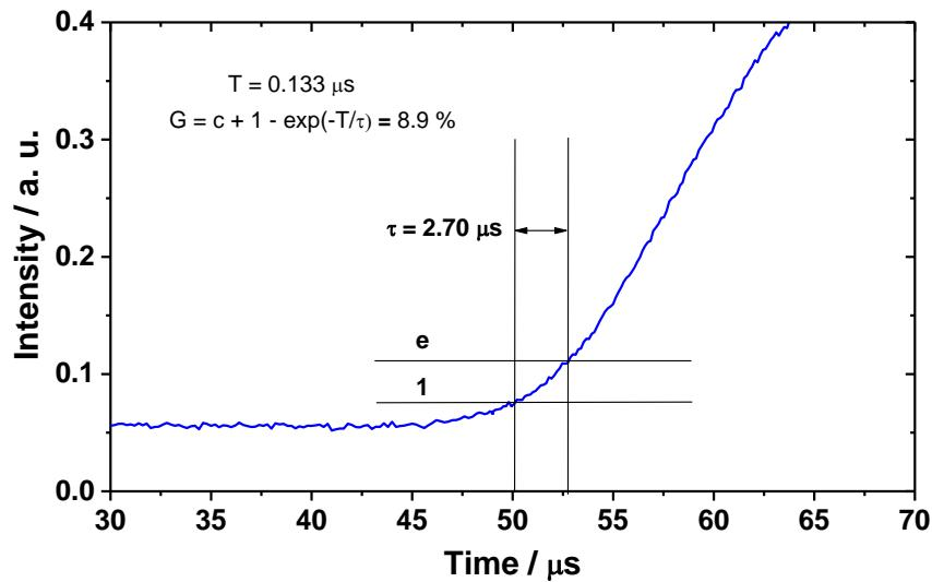
**Figure S12.** Gain calculation for the second FEL. The signal envelope was obtained by FindPeaks function of Wolfram Mathematica 10. Characteristic exponential time is  $2.70 \mu\text{s}$ .
