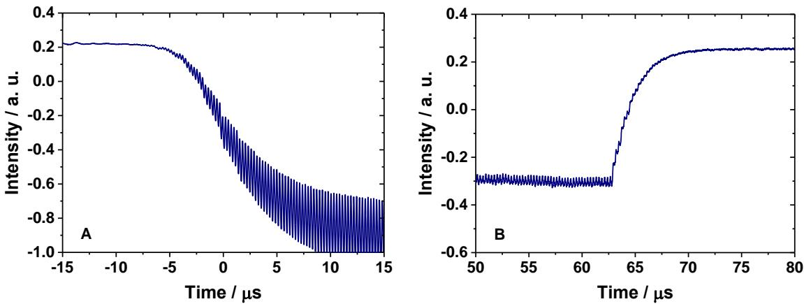
**Figure S7.** (A) The rising edge of the macropulse with  $100\text{ }\mu\text{s}$  duration; (B) The falling edge of another macropulse with  $100\text{ }\mu\text{s}$  duration. No pick-up coil synchronization was used for B.
