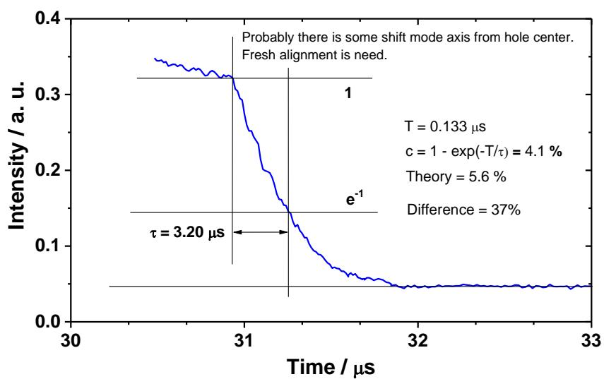
**Figure S11.** Calculation of losses for the second FEL. The signal envelope was obtained by FindPeaks function of Wolfram Mathematica 10. Characteristic exponential time is 3.20  $\mu\text{s}$ .
