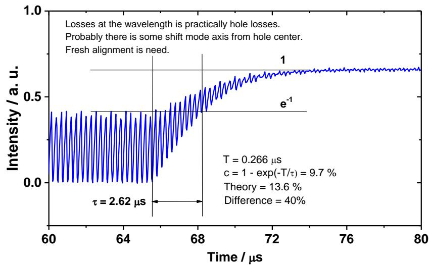
**Figure S13.** Calculation of losses for the third FEL. Characteristic exponential time is  $2.62 \mu\text{s}$ .
