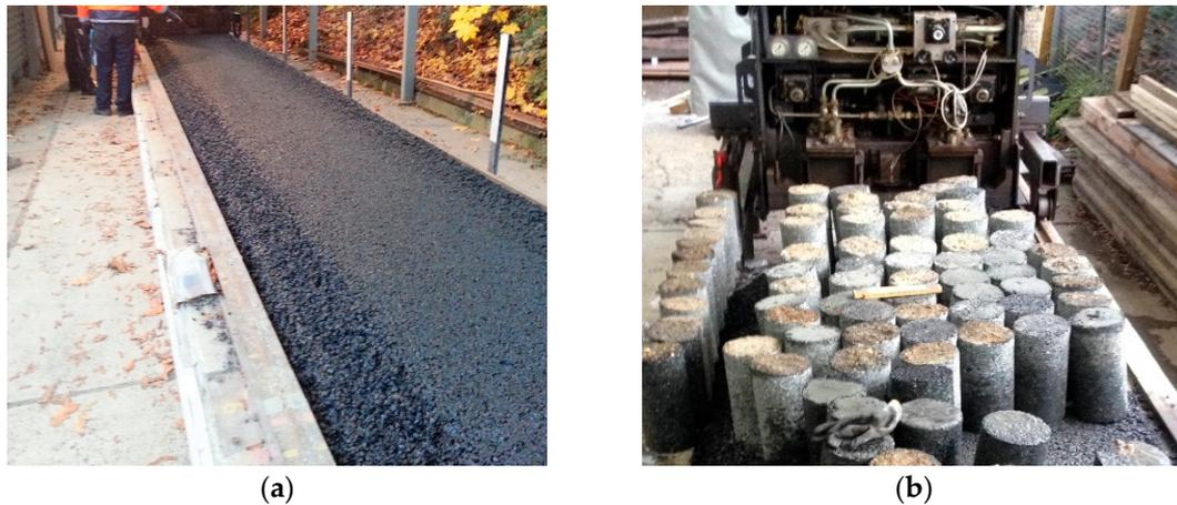
**Figure 2.** The preparation of the asphalt specimens. (a) Test track. (b) Cylindrical cores.
