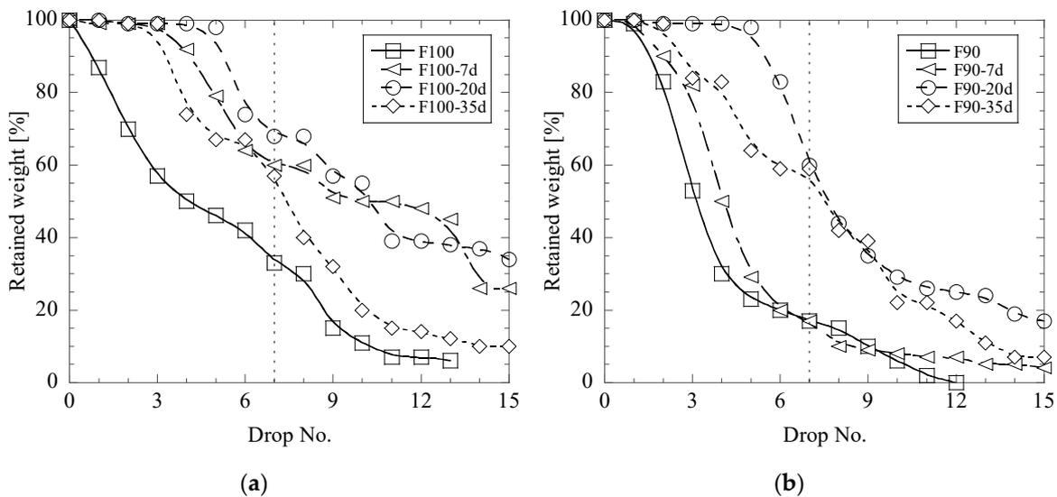
Figure 4. Effect of storage of briquettes F100 (a) and F90 (b) in air on the retained weight during drop test trials.
