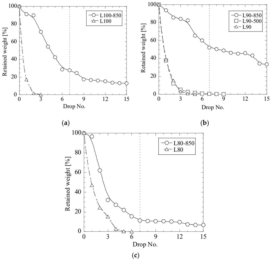
Figure 6. Relationships between retained weight of briquettes L100 (a), L90 (b) and L80 (c) and drop number in drop test trials for different lime mud briquettes before and after heat treatments at 500 °C and 850 °C.
