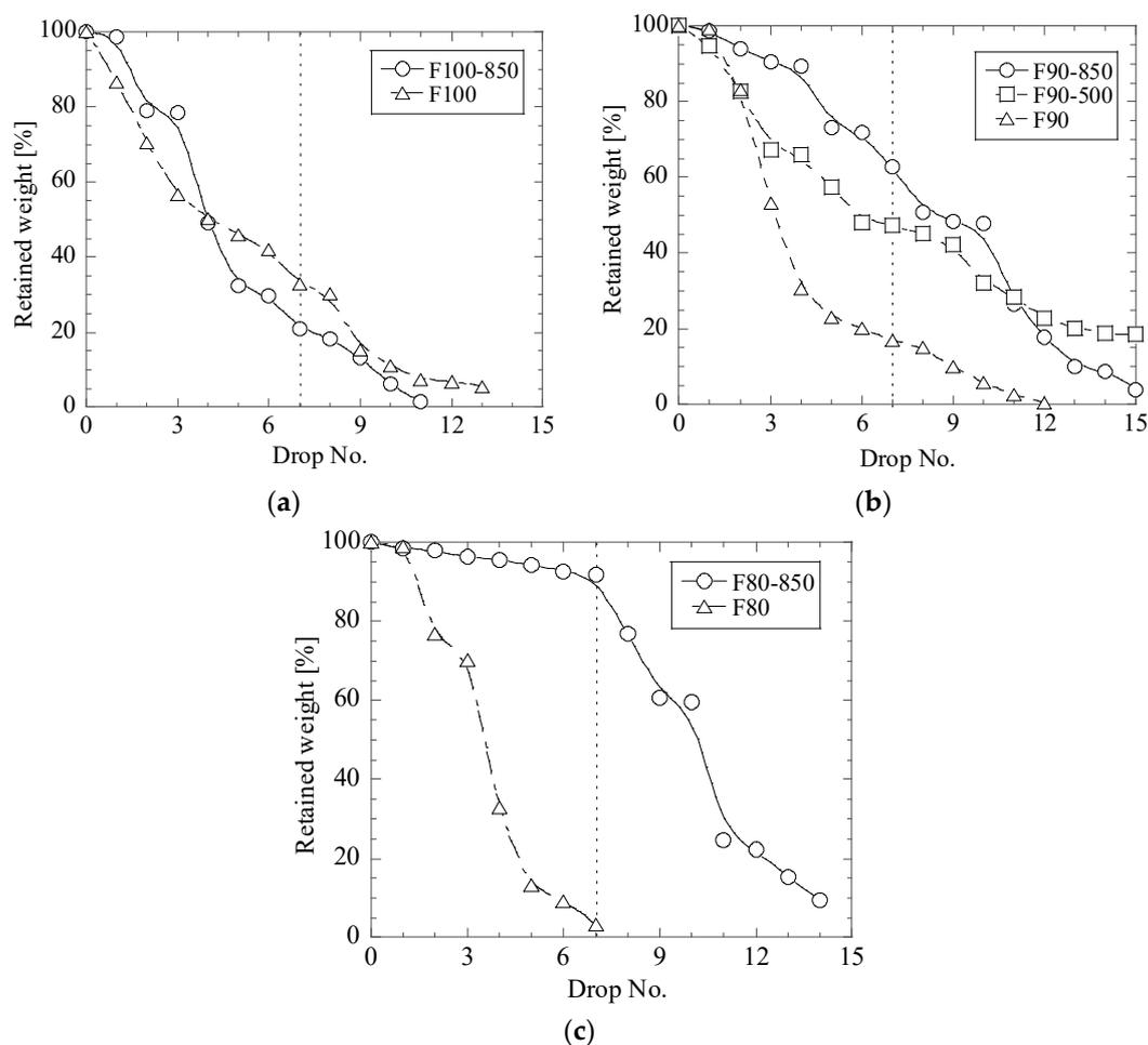
**Figure 7.** Relationships between retained weight of briquettes F100 (a), F90 (b) and F80 (c) and drop number in drop test trials for different fly ash briquettes before and after heat treatment at 500 °C and 850 °C.
