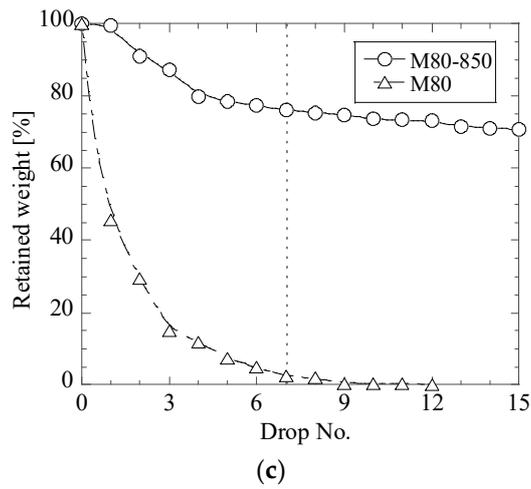
Figure 5. Relationships between retained weight of briquettes M100 (a), M90 (b) and M80 (c) and drop number in drop test trials for mesa briquettes before and after heat treatment at 500 °C and 850 °C.
