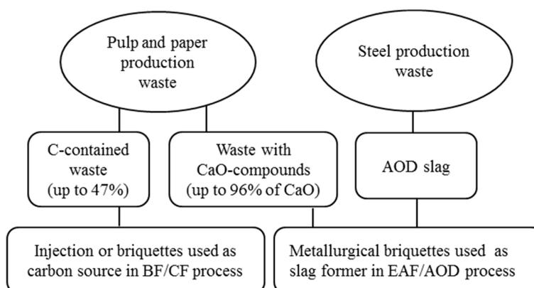
**Figure 2.** Application of wastes from pulp and paper industries in metallurgical processes.
