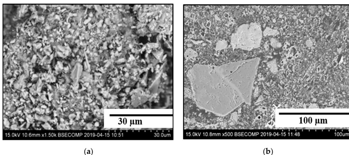
**Figure 9.** Typical scanning electron microscopy (SEM) images of small particles (a) and large blocks (b) in investigated powders and briquettes.
