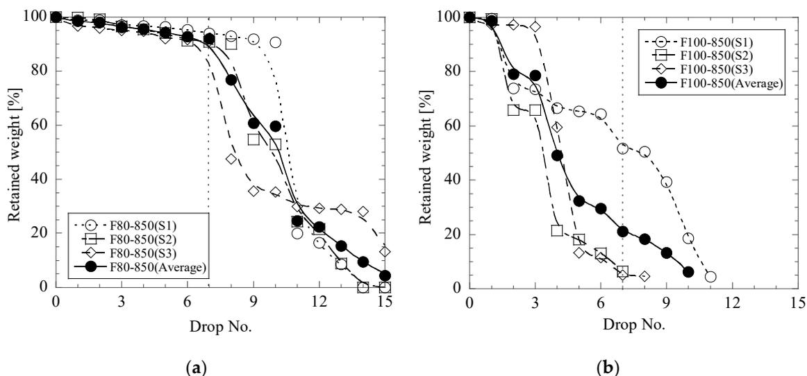
**Figure 3.** Relationships between retained weight of briquettes and drop number in drop test trials for briquettes of F80-850 (a) and F100-850 (b).
