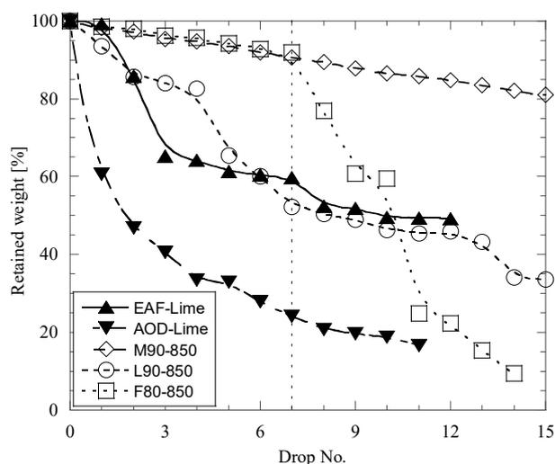
**Figure 8.** Comparison of drop test results for the best metallurgical briquettes (M90-850, L90-850 and F80-850) and lime lumps for electric arc furnaces (EAF) and argon oxygen decarburization (AOD) converter.
