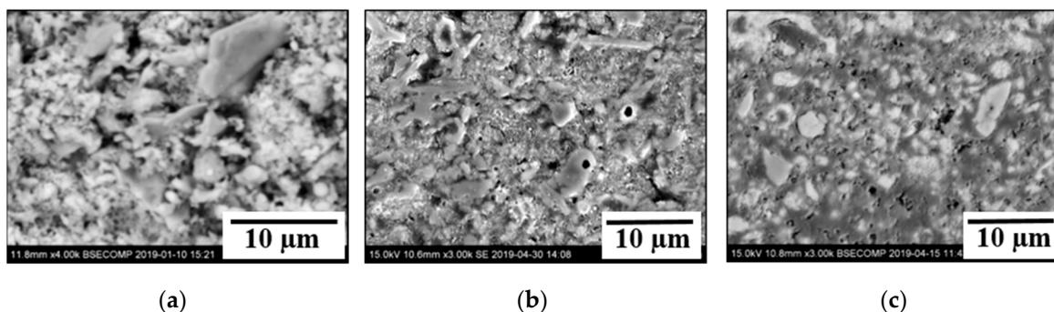
**Figure 10.** Typical SEM images of small particles in fly ash powder (a) and in F80 briquettes before (b) and after (c) heat treatment at 850 °C.
