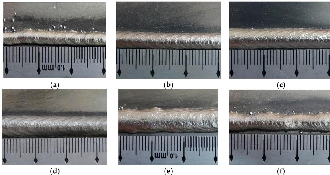
**Figure 5.** The appearance of the weld bead. (a) Specimen I1, (b) specimen I2, (c) specimen I3, (d) specimen I4, (e) specimen I5, (f) specimen I6.
