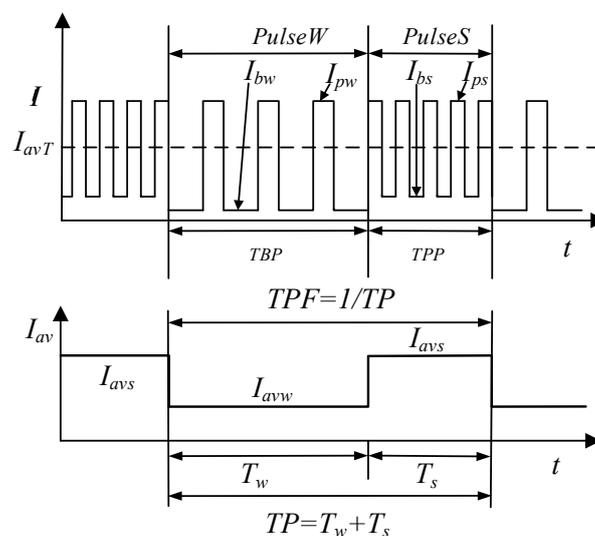
**Figure 1.** Schematic representation of current pulses during the double-pulsed gas metal arc welding (DP-GMAW) process.
