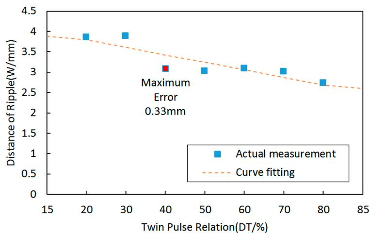
**Figure 12.** The variation tendency between distances of ripples and twin pulse relation and the curve fitting result.
