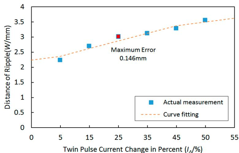
**Figure 14.** The variation tendency between distances of ripples and twin pulse current change in percent and the curve fitting result.
