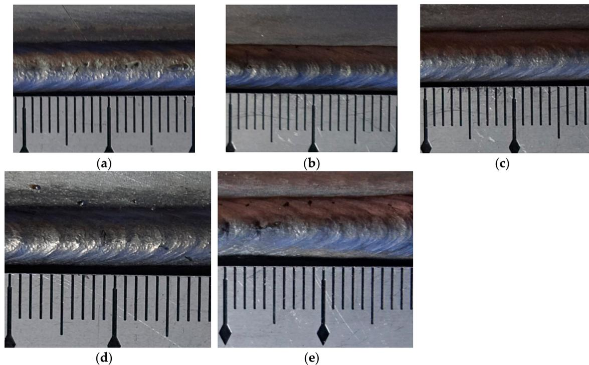
**Figure 15.** The appearance of the weld bead. (a) Specimen Y1, (b) specimen Y2, (c) specimen Y3, (d) specimen Y4, (e) specimen Y5.
