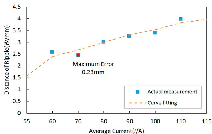
**Figure 6.** The variation tendency between distances of ripples and the average currents and the curve fitting result.
