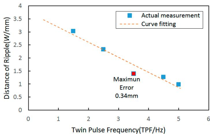
**Figure 10.** The variation tendency between distances of ripples and twin pulse frequency and the curve fitting result.
