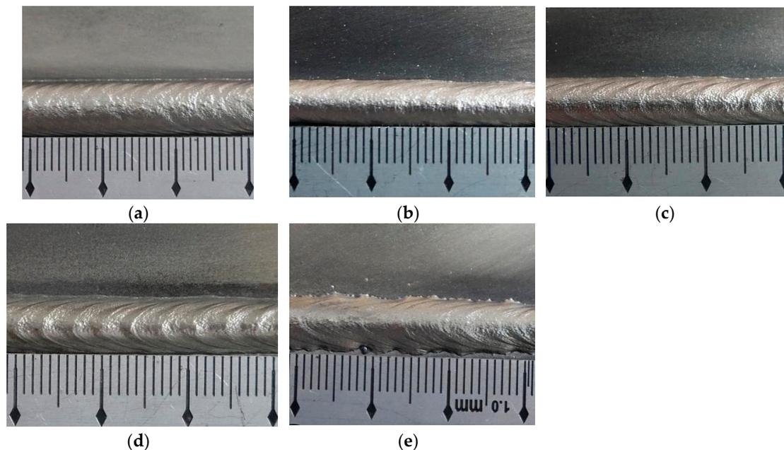
**Figure 13.** The appearance of the weld bead. (a) Specimen CC1, (b) specimen CC2, (c) specimen CC4, (d) specimen CC5, (e) specimen CC6.
