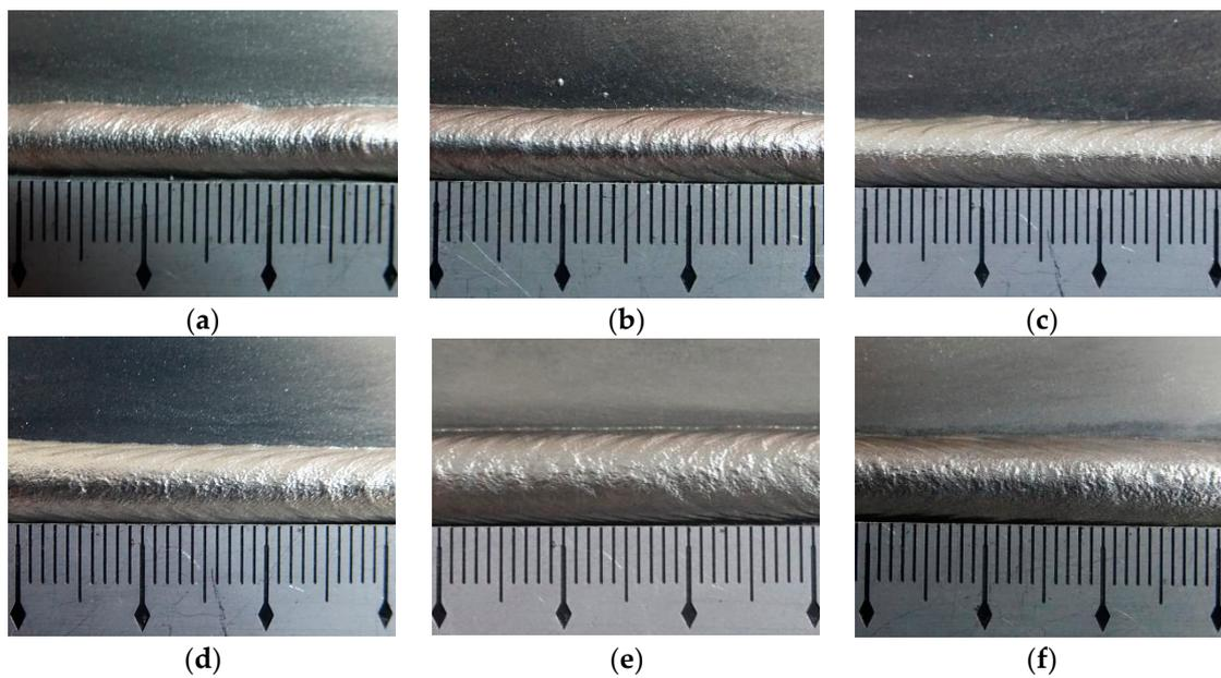
**Figure 11.** The appearance of the weld bead. (a) Specimen R1, (b) specimen R2, (c) specimen R3, (d) specimen R5, (e) specimen R6, (f) specimen R7.
