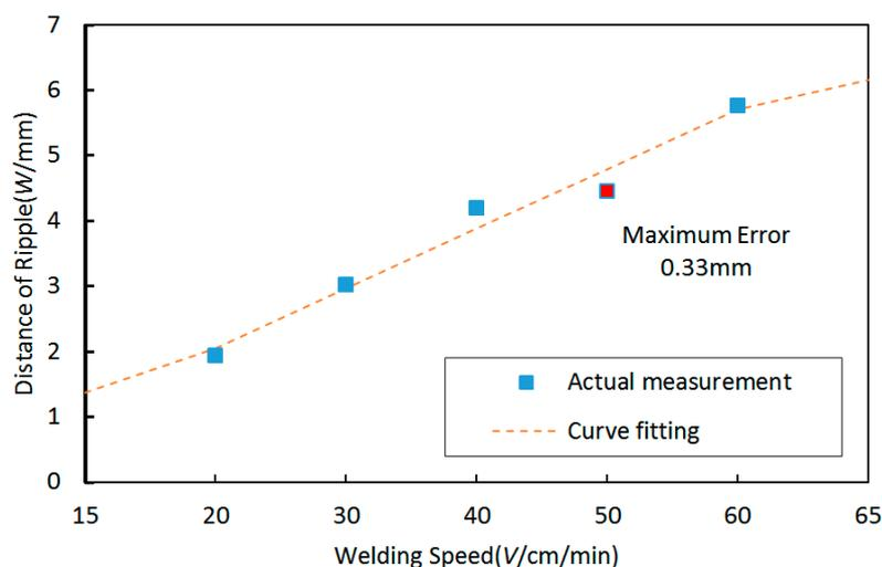
**Figure 8.** The variation tendency between distances of ripples and welding speed and the curve fitting result.
