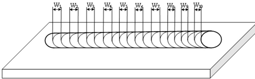
**Figure 4.** The schematic representation of the second measurement method of the distance of the ripples.
