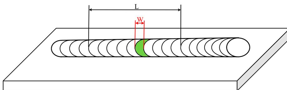
**Figure 3.** The schematic representation of the distance of ripples and the first measurement method.
