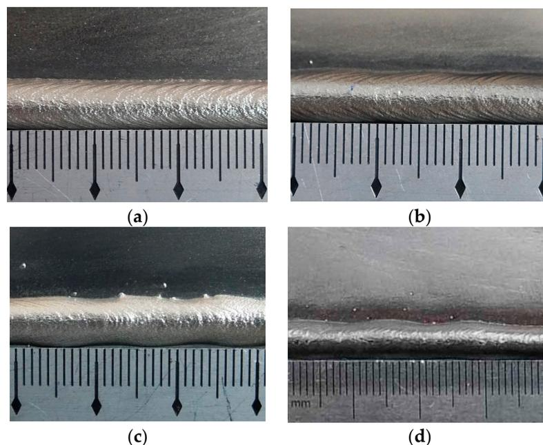
**Figure 9.** The appearance of the weld bead. (a) Specimen F2, (b) specimen F3, (c) specimen F4, (d) specimen F5.
